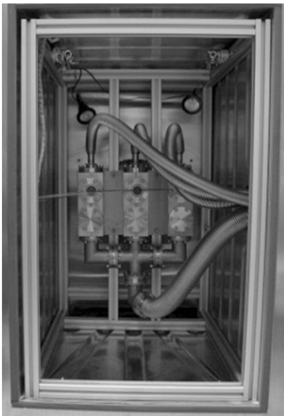
Figure 4. Humidity measurement cells inside the Temperature Test Chamber.
