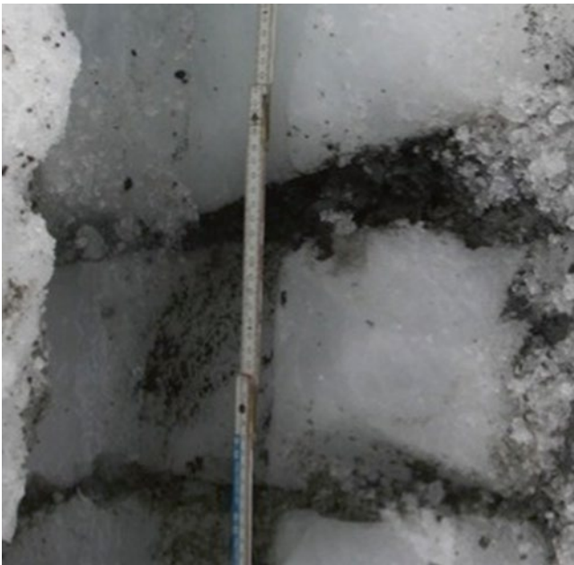
Figure 12. Third channel, 45^\circ downwards, \approx 3 m, penetration of \approx 4 cm of “dirt” (dust/sand/grit found on the glacier).
