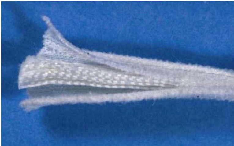
Fig. 7. Stryker-Meadox Dacron implant. The outer velour sheath has been opened to show the dense load-bearing Dacron tapes in the interior.
