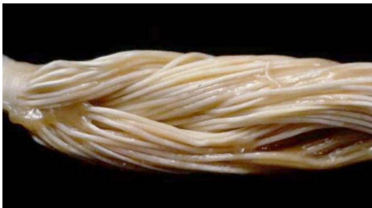
Fig. 4. Gore-Tex PTFE implant retrieved after 6 yr, indicating plaited structure and minimal tissue integration.
