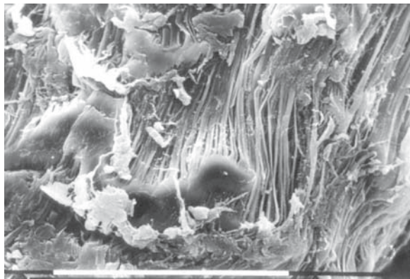
Fig. 6. Scanning electron micrograph of Gore-Tex implant, illustrating microfilaments of PTFE linking the solid nodes ( \times 570 magnification).
