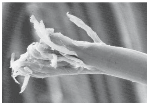
Fig. 13. Scanning electron micrograph of damaged polyester filament from ruptured implant ( \times 1400 magnification).
