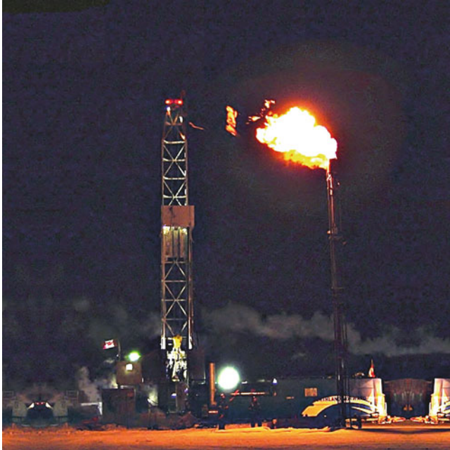
Fig. 6 Gas flare from the thermal gas hydrate production test in the Mallik 5L-38 gas hydrate research well (photo courtesy of the Mallik 2002 Gas Hydrate Production Research Well Program [35])
