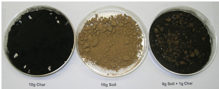
Fig. 3 Photographs showing, from left to right , 10 g biochar from pyrolysis of cornstover, 10 g soil, and 10 g mixture of biochar (10% W) and soil (90% W). The soil sample shown here is a surface soil from 0 to 15 cm deep at the University of Tennessee’s Research and Education Center, Milan, Tennessee, USA (358,560 N latitude, 888,430 W longitude), which is also known as the Carbon Sequestration in Terrestrial Ecosystems site (CSiTE) supported by the US Department of Energy (reproduced from ref. [5])
