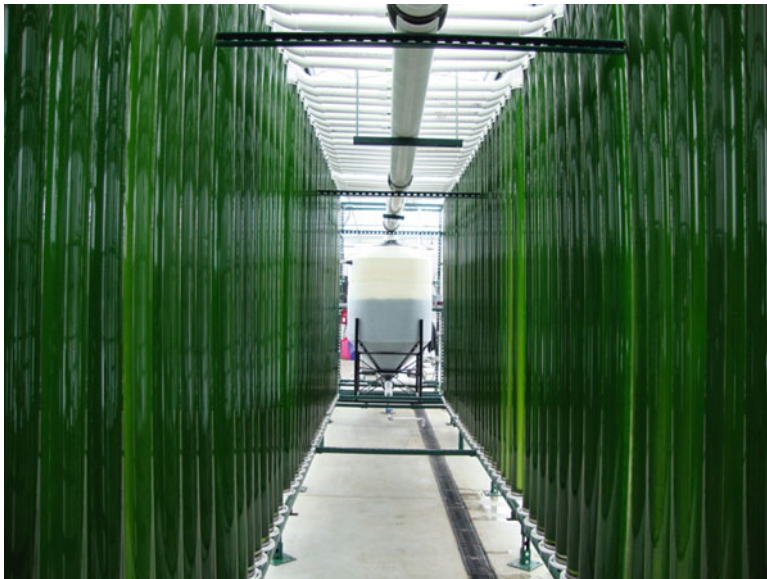
Fig. 6 A 400-litre vertical column photobioreactor in operation (Photo courtesy of Centre for Applied Energy Research, University of Kentucky, Lexington, KY, USA)
