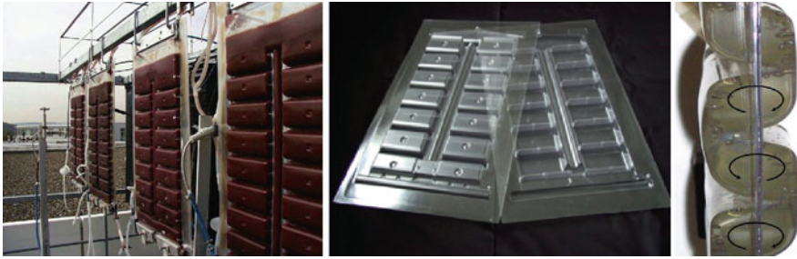
Fig. 9 Flat panel airlift reactor developed by Subitec (Stuttgart, Germany). Left : Outdoor cultivation with the flat panel airlift reactor. Middle : Forefront and backside of the reactor with characteristic slots and baffles. Right : Circular liquid flow through illuminated and dark zones is induced by the specific design with static mixers
