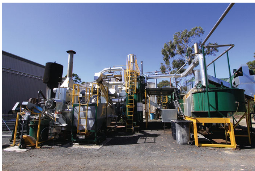
Fig. 3 Pacific Pyrolysis Pty Ltd's slow-pyrolysis demonstration facility at Somersby, Australia. Production facility for Agrichar™ biochar and bioelectricity from syngas
