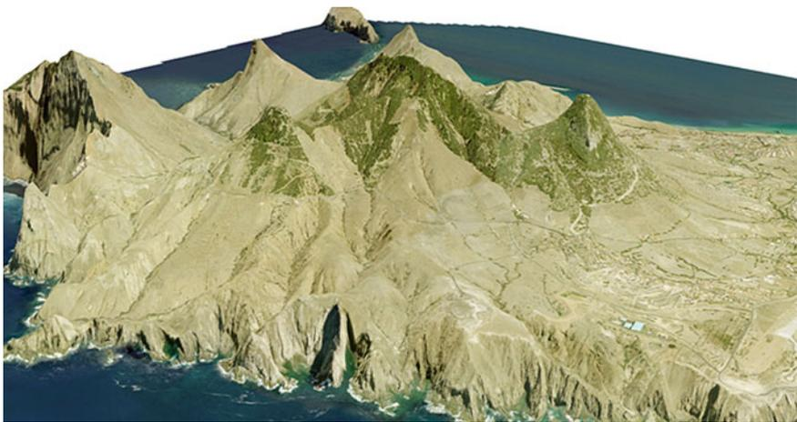
Fig. 4.41 Perspective representation of a DTM with draped orthoimage (Porto Santo Island)
