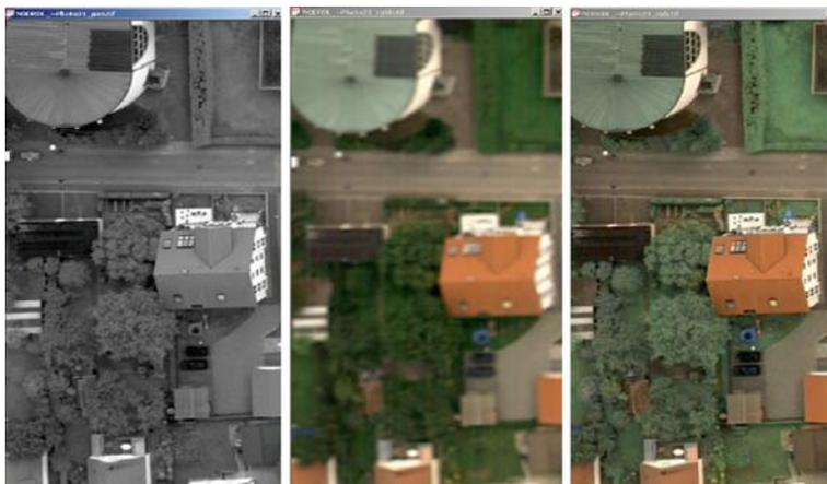
**Fig. 4.10** Obtaining a colour image (*right*) through pan-sharpening (Intergraph)
