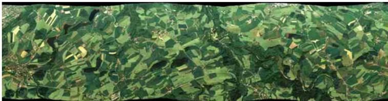
**Fig. 4.7** A RGB composite image acquired with an ADS camera and corrected from attitude variation (Leica Geosystems)
