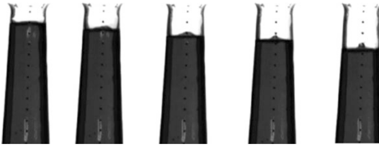
Fig. 7 Sequence of pictures showing an early time of the experiment. A nipple at the middle part of the free surface was observed
