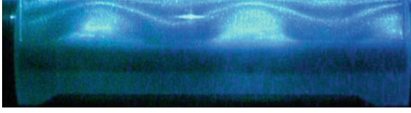
Fig. 3 Visualization of the elliptical instability of a tidally distorted deformable rotating cylindrical shell. In this illustration, the unstable mode is oscillating at a pulsation equal to \Omega and corresponds to a resonance between two Kelvin waves with azimuthal wavenumbers 0 and 2
