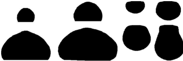
Fig. 5 Generated bidimensional profiles from photos obtained experimentally from drops which emerge downwards and upwards. They were used to find centers of mass, volume and area
