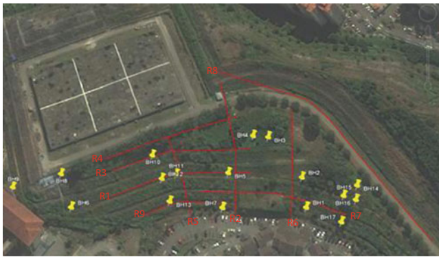
Fig. 2 Location of boreholes and resistivity survey lines
