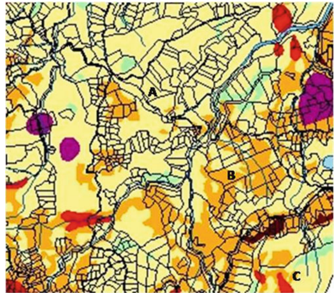
Fig. 2 A part of a landslide hazard zonation map showing a land parcel that belong to one hazard zone (A), a land parcel that belong to two hazard zones (B), a land parcel that belong to several hazard zones (C)
