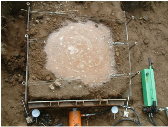
Fig. 5 Horizontal push-shear in-situ test of saturated accumulation body
