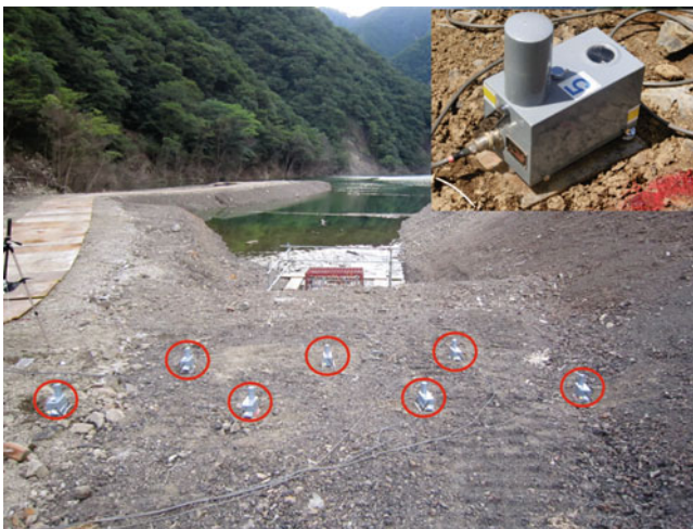
Fig. 10 Chain array method of geophone arrangement at station D–D' on Akatani landslide dam (geophone inserted at the top right corner)
