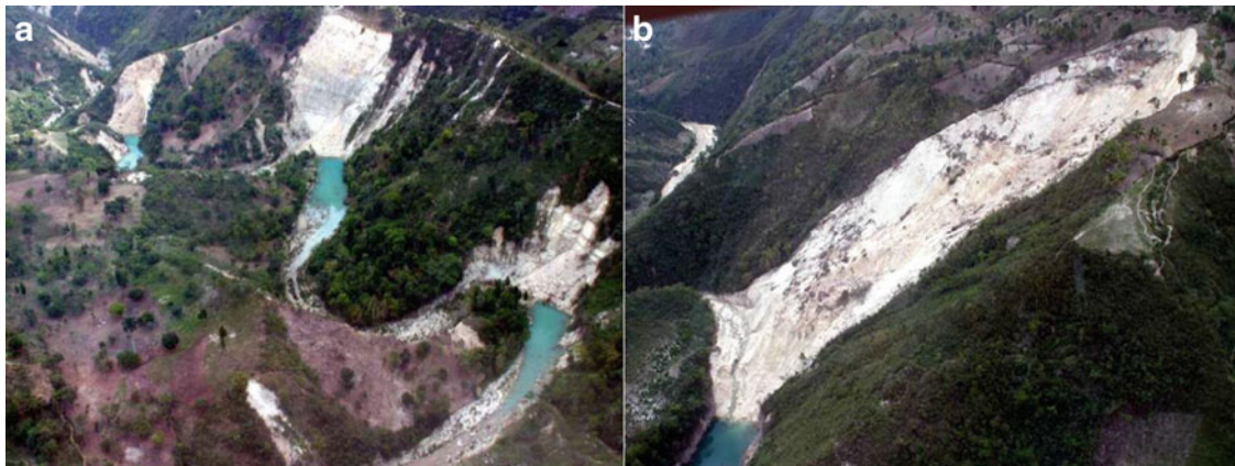
Fig. 3 Photos taken from helicopter (Jibson and Harp 2011). (a) Several landslides dams resulted in beaded dammed lake; (b) a typical landslide dammed a drainage
