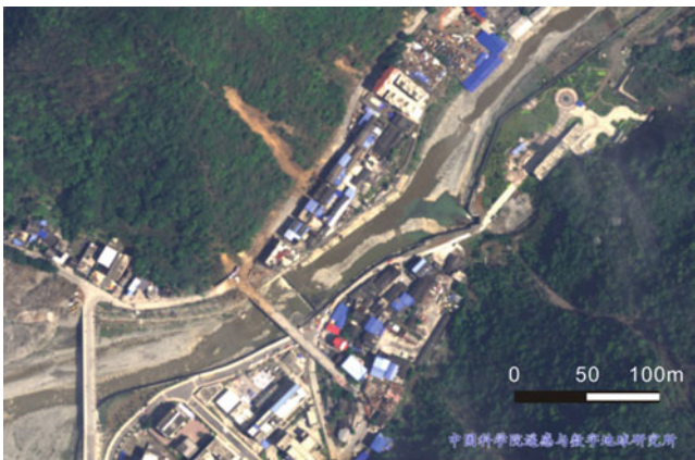
Fig. 5 Less than 300 m, more than two landslides have been found along the regional road S210 in Baoxing County
