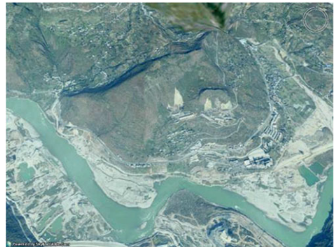
Fig. 8 Aerial image of landslide area, the gentle topography of landslide area and isolate rock mass in Zone B are both clearly classified
