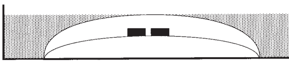
Fig. 1. Schematic diagram of a three-dimensional collagen gel culture. Side view, showing explants positioned at the interface between the collagen bilayer. The explants should lie in the center of the gel and rest on the bottom collagen cushion. The bottom layer of collagen is flat. The top layer of collagen overlays the bottom cushion precisely. Medium is added just to cover the gel.
