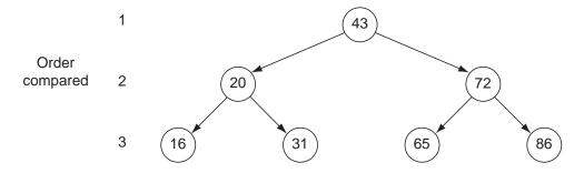
Observe that for each key K in this tree, all of the keys in K's left subtree are less than K and all of the keys in K's right subtree are greater than K. Trees with this property are referred to as binary search trees.
