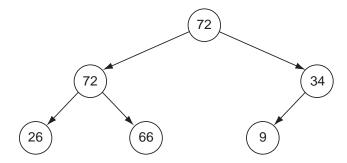
The fact that the tree is complete means that a heap can be stored in level order in an array without introducing gaps (unused areas) in the middle. The result is a compact representation in which you can easily move up and down the branches.
