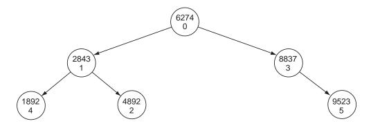
Given an account ID, retrieval of the corresponding account record is a two-step process. First, you retrieve the data item from the index tree that has the specified account ID. Then, using the record number stored in the index data item, you read the corresponding account record from the database file. The result is an efficient retrieval process that is based on account ID.
