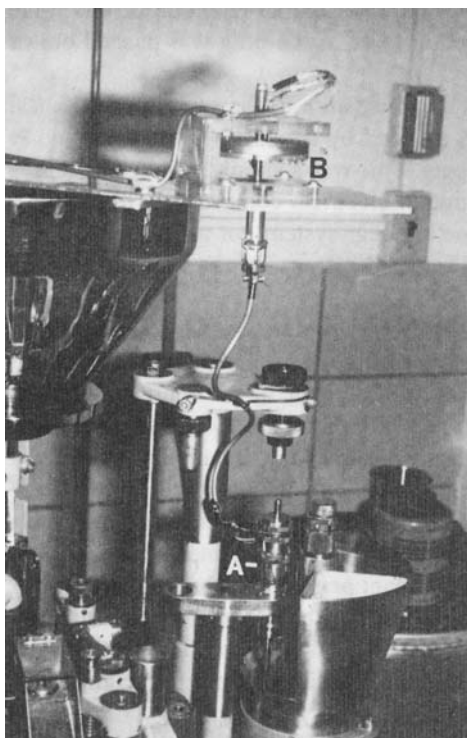
Fig. 15 Instrumented Zanasi LZ-64 showing mercury swivel for signal removal: (A) dosator containing strain-gauged piston; (B) mercury swivel. (From Ref. 38.)
