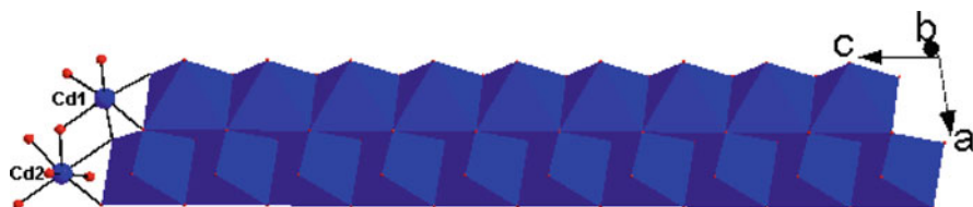
Fig. 22 1D chain formed by Cd1O 6 and Cd2O 7 polyhedra within Cd 4 BiO(BO 3 ) 3
