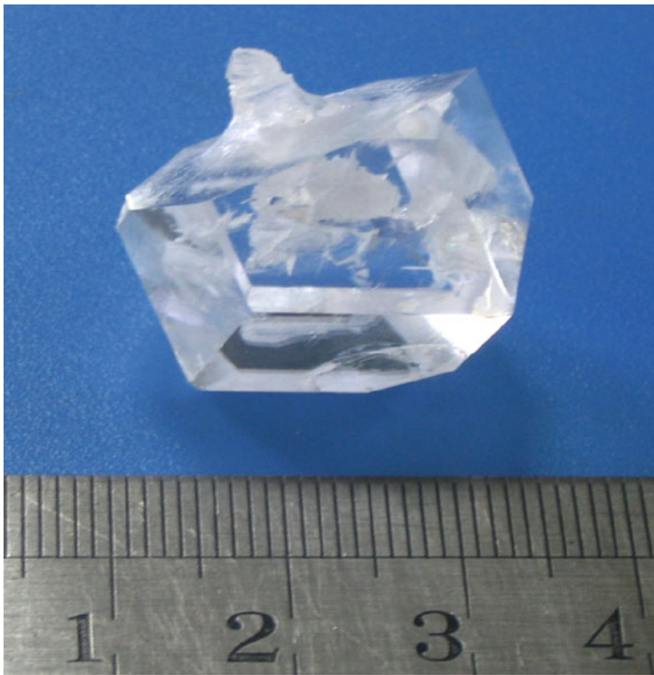
Fig. 2 As-grown YLSB crystal
