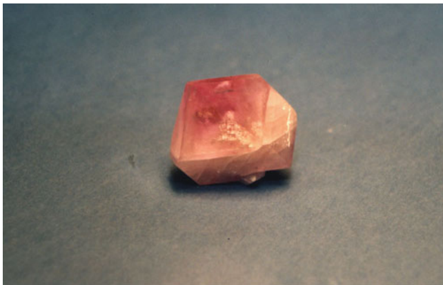
Fig. 4 \text{Ti}^{3+}:\text{YAl}_3(\text{BO}_3)_4 crystal with dimension 42 \times 36 \times 24 \text{ mm}^3 grown by TSSG method from flux of \text{K}_2\text{Mo}_3\text{O}_{10}\text{-B}_2\text{O}_3 [43]
