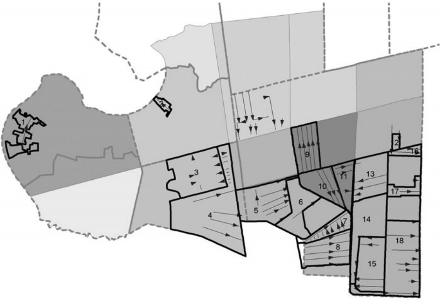
Figure 10-11. Service areas, flow directions, and main outlets in the project area.
