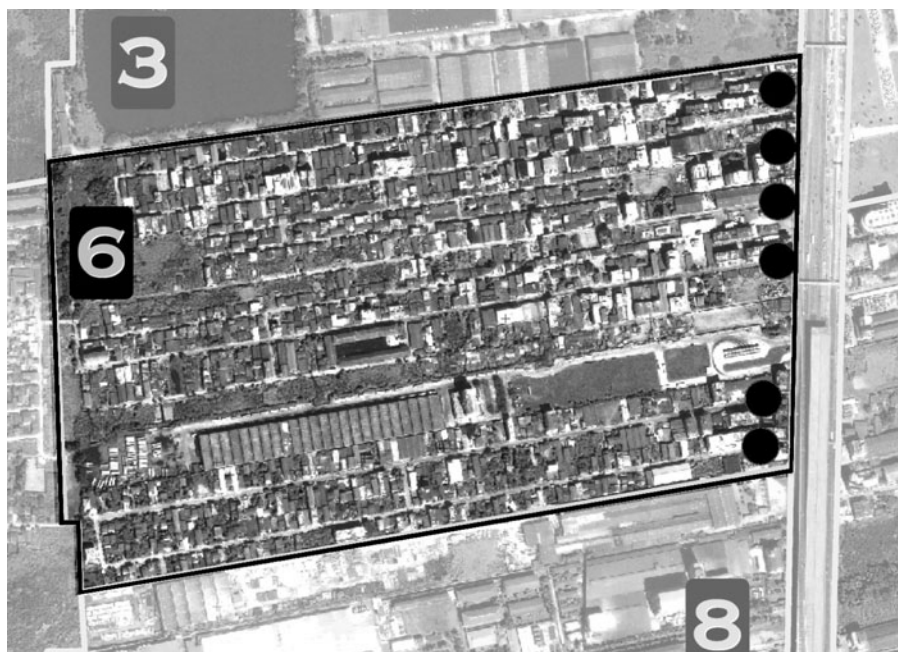
Figure 10-10. Option 3: location of mini-treatment plants (black dots) for a key area within the catchment.
