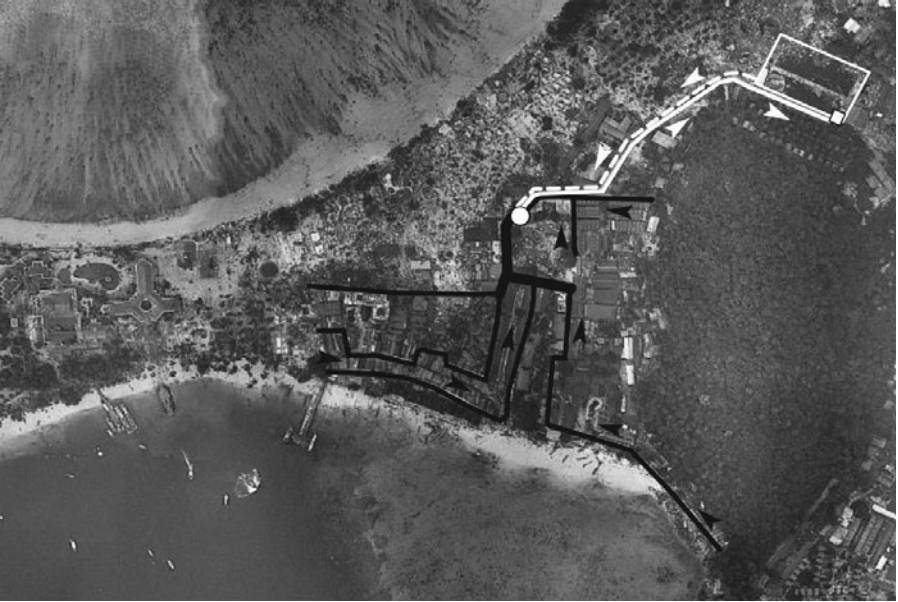
Figure 6-5. The wastewater collection system with secondary pipes ( black ), mains ( bold black ), pressure pipe ( white ), re-use water pipe ( dashed white ), pumping station ( round dot ), and inlet structure ( square dot ).
