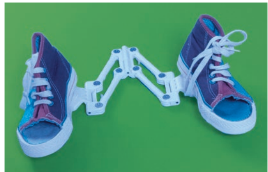
Fig. 16.15 Contrarotational system. The shoes can be adjusted with respect to the frame. In an internal rotation of the lower legs the shoes will be turned outwards 20° in a few steps
