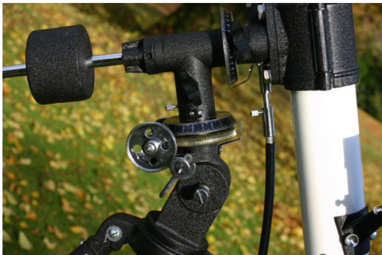
Fig. 6.3 The Tasco 14TE mount is light but sturdy. It is heavily greased, and you can see it (Image by the author)
