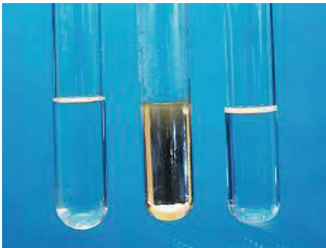
Fig. 7.7 A thin deposit of silver forms when a reducing agent is added to Tollen's reagent
