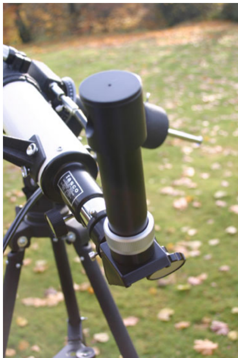
Fig. 6.17 A good way to check initial collimation—just add an inexpensive Cheshire eyepiece (Image by the author)
