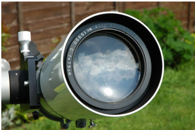
Fig. 4.3 Zeiss also produced rich field refractors such as this 110 mm f/7 achromat (Image credit: Richard Day)
