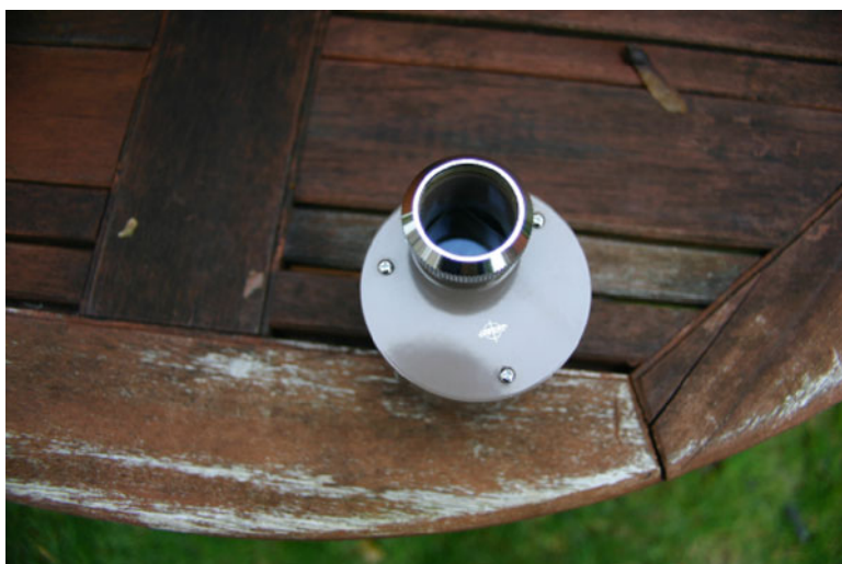
Fig. 6.11 Another nice Swift touch—a high quality terrestrial viewer can be added for day-time observing (Image by the author)
