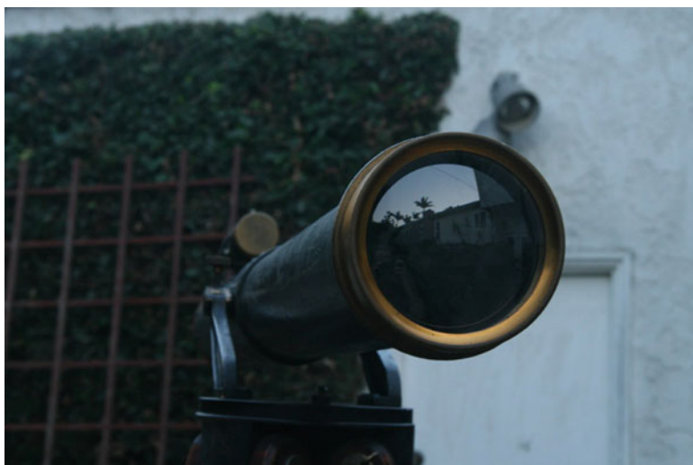
Fig. 3.18 Brashear often employed a Steinheil-like approach to building his object glasses. This 4-in. Brashear achromat has a flint leading element
