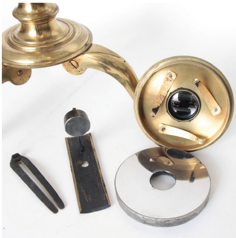
Fig. 7.4 The innards of a Gregorian telescope by George Adams, Sr (Image credit: Fleaglass.com)
