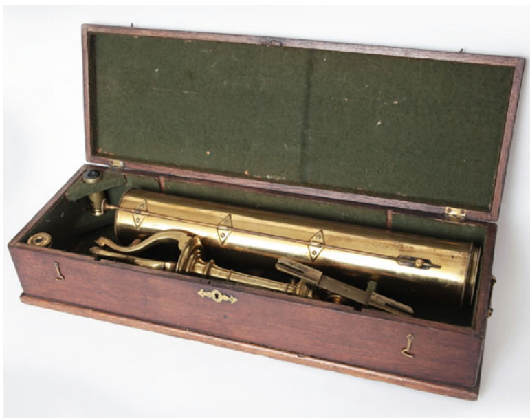
Fig. 7.3 A 4-in. reflector with mount and eyepieces made by George Adams, Sr (Image credit: Fleaglass.com)
