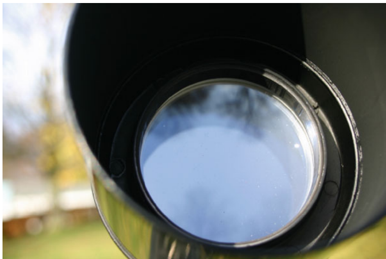
Fig. 6.12 The 14TE has an air-spaced doublet objective, though it's hard to tell until you take a closer look inside. \text{MgF}_2 coatings were applied to inner and outer surfaces (Image by the author)
