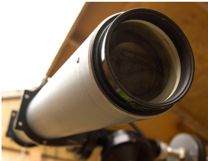
Fig. 4.4 The Steinheil doublet objective of the Zeiss AS80 (Image credit: Pat Conlon)
