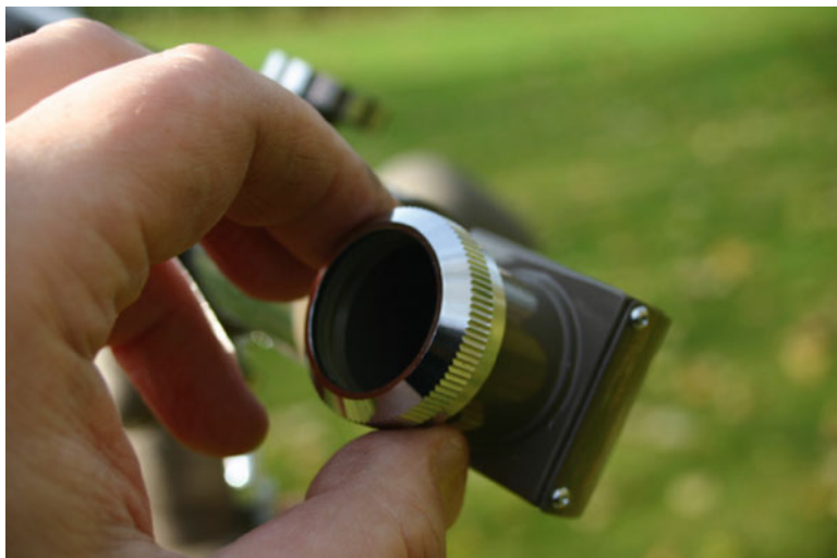
Fig. 6.15 Check out this little piece of engineering magic. The Swift comes with a precision made prism diagonal and a lovely helical eyepiece grip (Image by the author)
