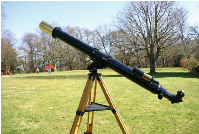
Fig. 2.13 In Amatam Memoriam : The author’s fine 4-in. f/15 refractor, inspired by the workshops of T. Cooke & Sons (Image by the author)
