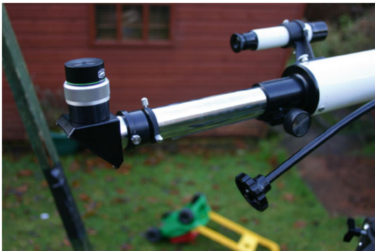
Fig. 6.19 The generous back focus on these small refractors makes them ideal as long distance microscopes (Image by the author)
