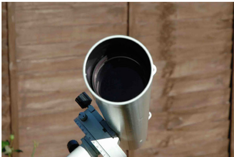
Fig. 4.8 The cemented achromatic doublet objective of the Zeiss Telementor (Image credit: Richard Day)
