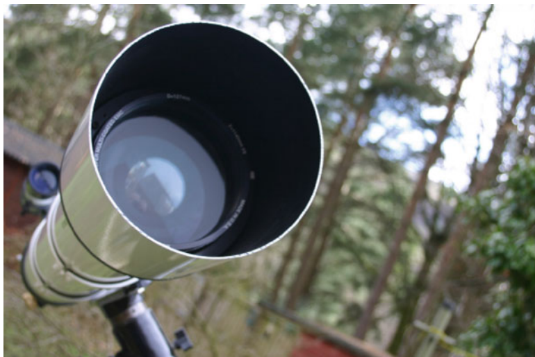
Fig. 10.2 The strong reflection from the uncoated low dispersion element of an early Meade 127 ED refractor (Image by the author)
