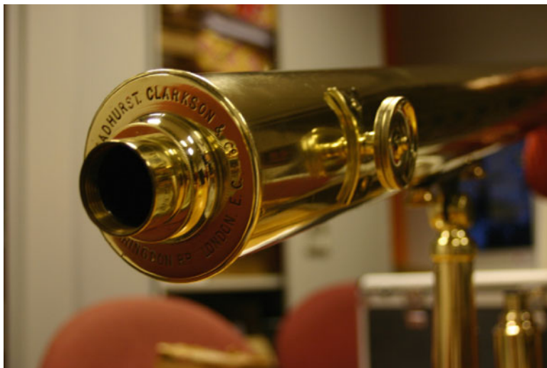
Fig. 12.3 Gleaming with pride – the exhaustively cleaned and polished optical tube (Image credit: Steve Collingwood)
