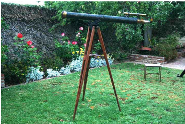
Fig. 3.16 A 4-in. f/15 Brashear achromat atop a stylish but sturdy alt-azimuth mount (Image credit: Dan Schechter)
