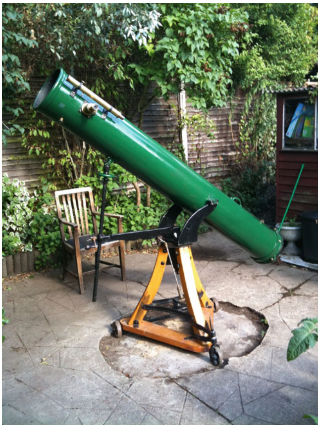
Fig. 7.8 A refurbished Calver reflector on an alt-az mount (Image credit: Robert Katz)
