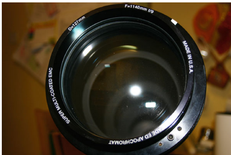
Fig. 10.9 Still performing well after nearly two decades of use, the Meade 127ED objective (Image by the author)
