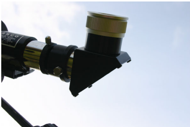
Fig. 6.14 An inexpensive adaptor enables me to use a high quality prism diagonal and my favorite 1.25-in. eyepieces (Image by the author)
