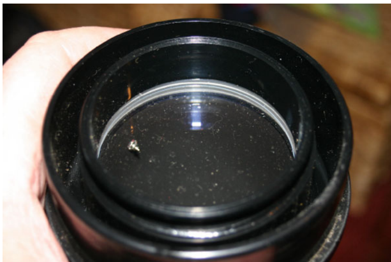
Fig. 6.24 Check out this botched job on the Tasco 58T! Note the plastic lens cell and protruding screw (Image by the author)
