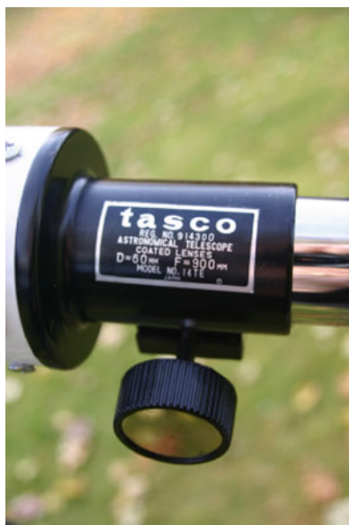
Fig. 6.7 The simple rack and pinion focuser on the 14TE. Check out the plastic focus knobs (Image by the author)
