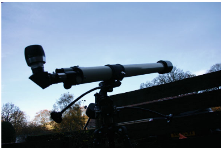
Fig. 6.21 The 14TE kitted out with a modern, wide-angle eyepiece works surprisingly well as a rich field ‘scope (Image by the author)
