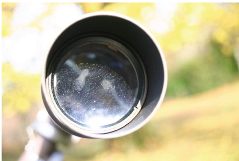
Fig. 6.13 The dusty Swift had an air-spaced doublet with all four surfaces coated with \text{MgF}_2 (Image by the author)
