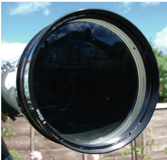
Fig. 10.4 The oil-spaced triplet objective on the 6-in. f/12 Starfire has weathered well after all these years (Image credit: Richard Day)
