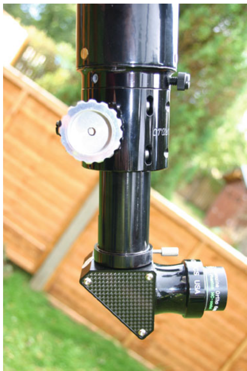
Fig. 6.28 Modern touches—the silky smooth Crayford of the Skylight f/15m (Image by the author)
