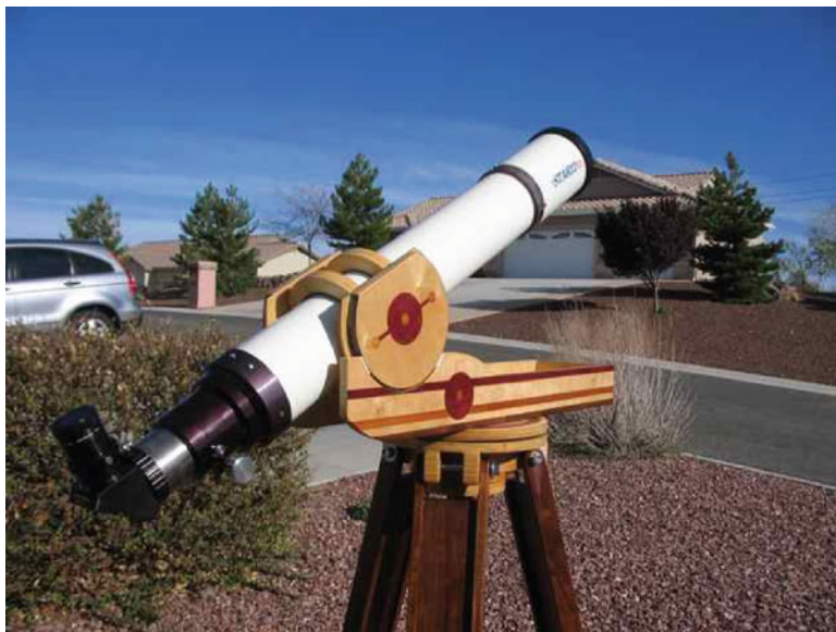
Fig. 10.6 The Astro-Physics Star12 on a homemade alt-az mounting (Image credit: Jeff Morgan)
