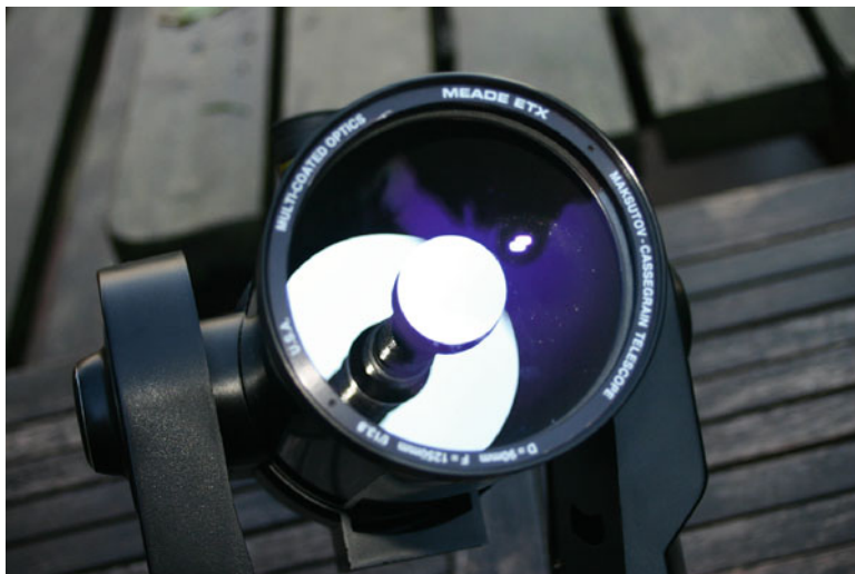
Fig. 11.7 The Maksutov Cassegrain design of the ETX offers up impressively sharp images when properly collimated (Image by the author)
