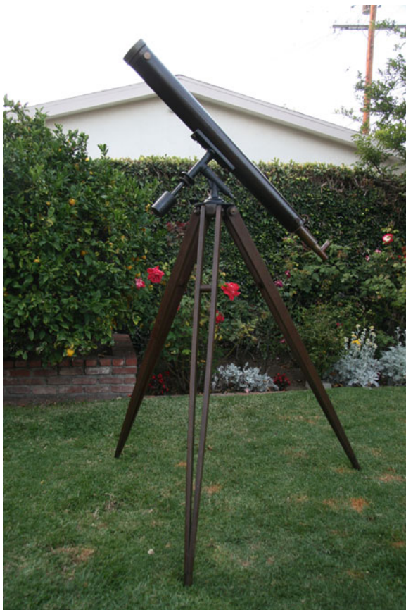
Fig. 3.6 A 4.13-in. Clark (c. 1860). Note the wooden tube (Image credit: Dan Schechter)
