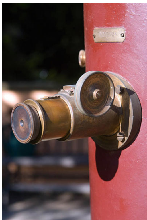
Fig. 7.11 The sturdy but supremely functional focuser on the Brashear reflector (Image credit: Dan Schechter)
