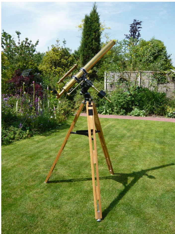
Fig. 5.8 A handmade c. 1910 3-in. Broadhurst-Clarkson ‘Starboy’ refractor (Image credit: Phil Jaworek)
