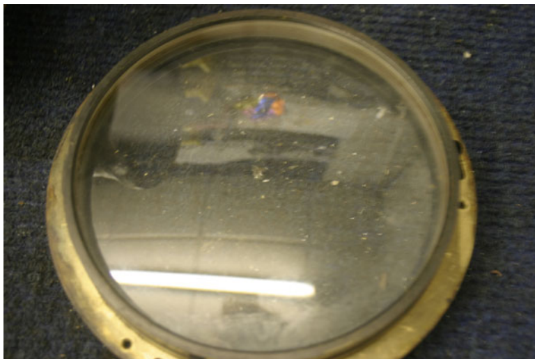
Fig. 12.10 The uncoated, late Victorian objective was in need of extensive cleaning but was otherwise pristine (Image credit: Steve Collingwood)
