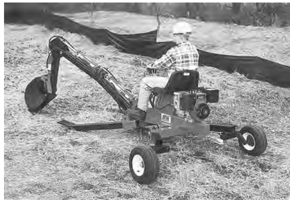
Figure 7.7 Not all machines need to be self-propelled. Trencherman backhoes, by NorthStar, are towed to work; the bucket levers the machine around the site. (Photo: Northern Tool and Equipment, manufacturer of NorthStar machinery.)
