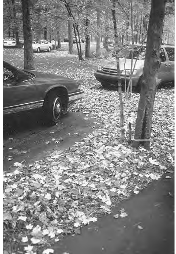
Figure 5.14 Dispersed parking for Simmons headquarters reduced disruption and infiltrates runoff near its source. ( Project: Robert Marvin Associates. Photo: Bruce Ferguson. )
