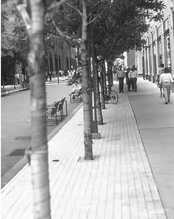
Figure 3.23 Continuous trench plantings can unify a streetscape. Paver joints are open to admit air and water. (Project and Photo: Henry Arnold.)
