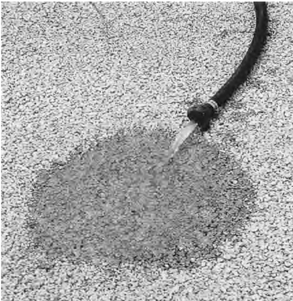
Figure 5.8 Porous concrete, shown here, and porous asphalt support vehicles but permit water to infiltrate rapidly. (Photo: Florida Concrete and Products Association/Dennis Graeber.)
