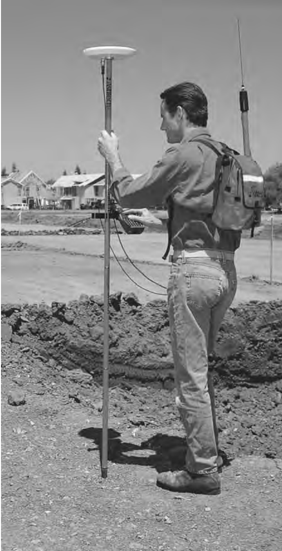
Figure I.4 GPS units, often backpack sized, make surveying quicker, easier, and potentially less destructive to site vegetation. (Photo: Magellan Corp. ☞)
