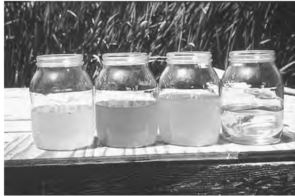
Figure 4.28 Increasing clarity is visible in water from Arcata CA’s constructed wetlands, sampled at progressive stages of wastewater treatment. From left: inflow to system; outflows from oxidation pond, treatment marsh, and enhancement marsh. (Photo: Professor Joe Meyer, University of Wyoming.)
