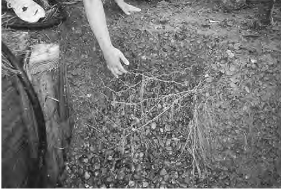
Figure 3.25a,b Structural soil resists compaction by incorporating crushed stone; soil fills voids, providing space for roots, air, and water. Diagram (b) shows components; paving over structure soil may be porous. (Photo: J. Grabosky.)
