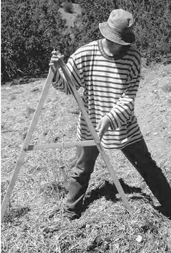
Figure I.5 The Egyptian A-frame is a simple, site-friendly way of establishing level and the fastest way to lay out points along a contour line. (Photo: Kim Sorvig.)
