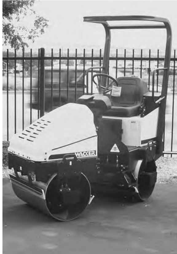
Figure 7.6 Articulated steering, as well as small size, means this roller can work around existing site features instead of obliterating them. (Photo: Kim Sorvig.)
