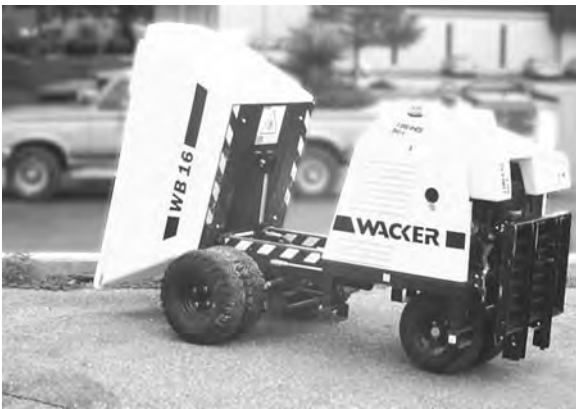
Figure 7.4 "Site dumpers" can be an efficient compromise between hand labor and full-size tractors. (Photo: Kim Sorvig.)
