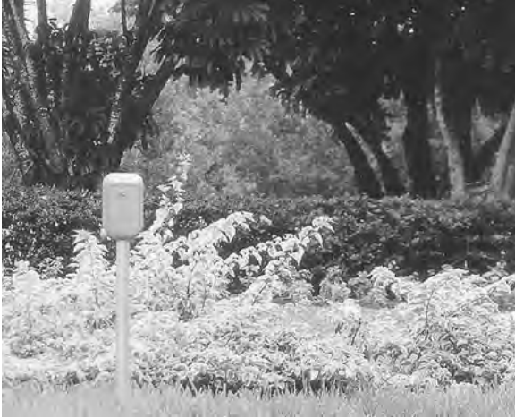
Figure 4.25 Small, solar powered, and radio controlled, LEIT irrigation controllers can save electricity as well as fuel used in site visits. (Photo: Altec Co. [now DIG Corp.] )
