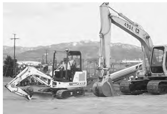
Figure 7.2 Some “heavy equipment” isn't. The small Bobcat excavator is about seven feet tall by three feet wide. Compared to the larger excavator shown, weight and fuel use are about 10 percent. (Photo: Kim Sorvig.)
