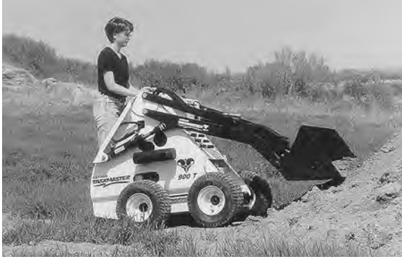
Figure 7.3 This mini skid steer, from Ramrod, fits where larger machines can't, and has an unusually wide range of attachments. Size generally corresponds to decreased fuel use and ground pressure. (Photo: Ramrod Equipment.)
