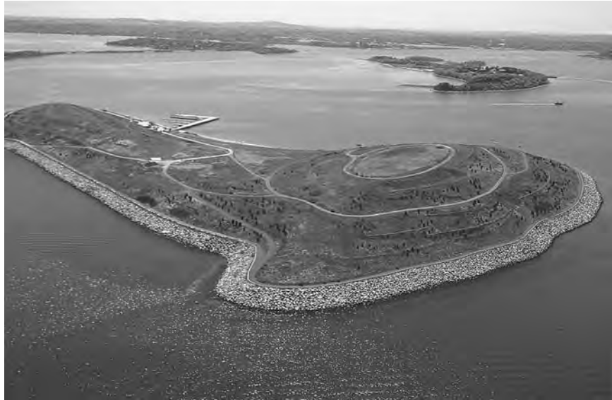
Figure 2.14 Spectacle Island in Boston Harbor is a recreational landscape salvaged from a toxic dump. (Project: P. Craul with Brown and Rowe. Photo: Massachusetts Turnpike Authority.)
