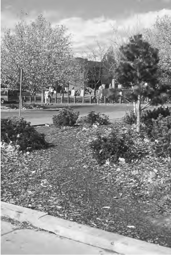
Figure 10.4 “Desire lines” occur at the point pedestrians see their destination. These lines can be counteracted by visual screening (barriers seldom work)—or they can be opportunities to link design to real-use patterns. (Photo: Kim Sorvig.)
