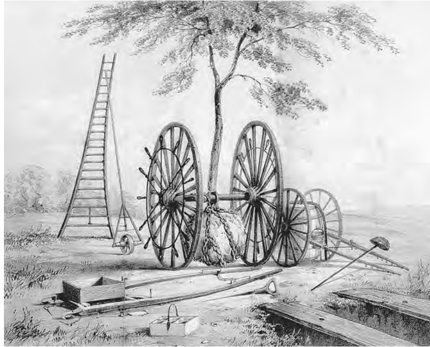
Figure I.I6 Col. Greenwood's Treelifter (1844) allowed one worker to transplant a thirty-foot tall tree. The "ship's wheel" cranked the axle, pulling up the lifting chains. In transit, the axle rotated independent of the chains. (Illustr.: From "The Tree-Lifter," London, 1844; thanks to Tim Brotzman, Brotzman's Nursery, Madison OH.)
