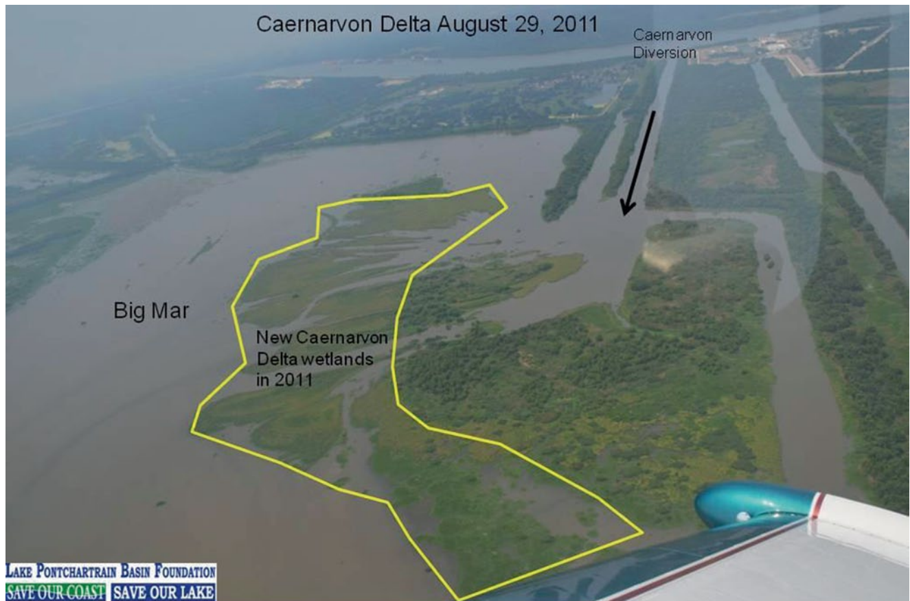
Fig. 5 Caernarvon Diversion showing Big Mar Lake receiving diversion flow, \sim 4 \text{ km}^2 of new wetlands have developed in the past decade (Courtesy Lake Pontchartrain Basin Foundation)
