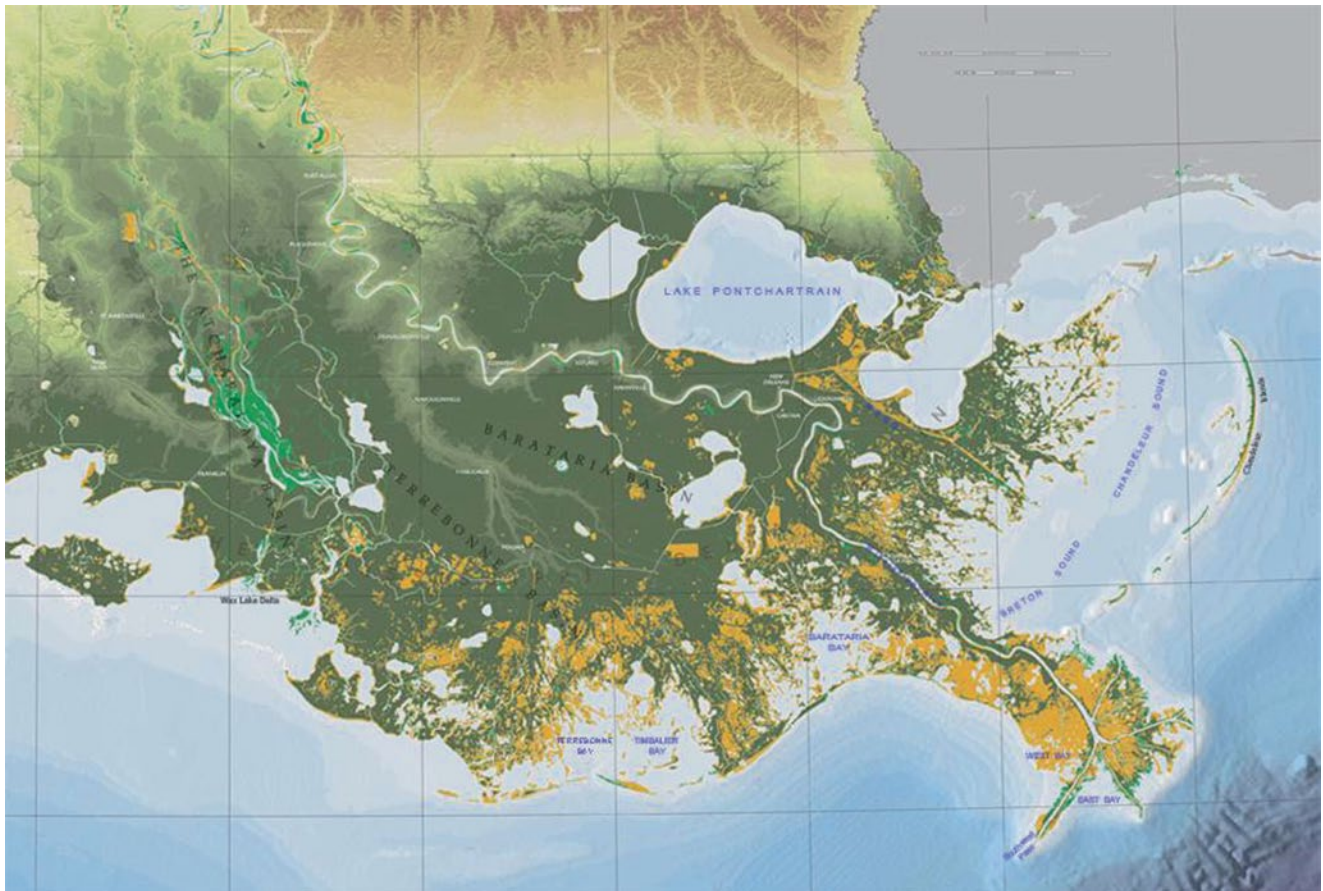
Fig. 2 Eastern Coastal Louisiana. Light green areas represent land gained 1937–2000; Orange areas represent land lost 1937–2000
