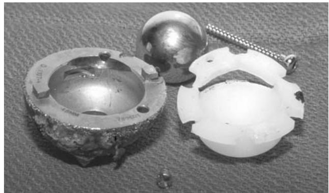
**FIGURE 2-20.** A 1-year conventional UHMWPE, primary acetabular liner demonstrating crack initiation and propagation. Failure initiated at a sharp edge of a locking point. (From Tradonsky, Postak, Froimson<sup>129</sup> by permission of *Clin Orthop*.)
