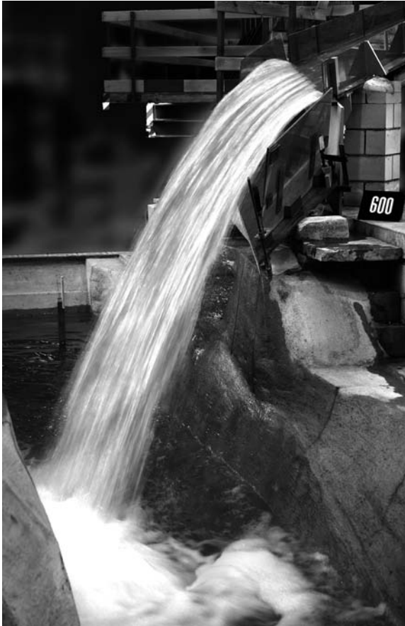
Figure 13.7 Kárahnjúkar dam model – jet and plunge pool (courtesy of VAW, ETH Zürich)
