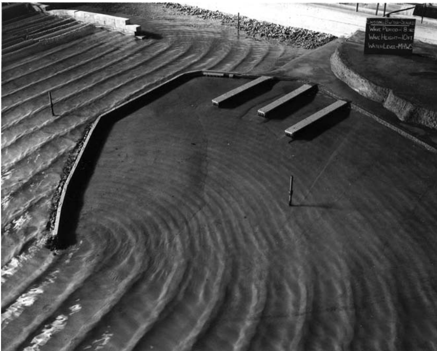
Figure 12.15 Model of a harbour with a breakwater and wave diffraction (courtesy of HR Wallingford)
