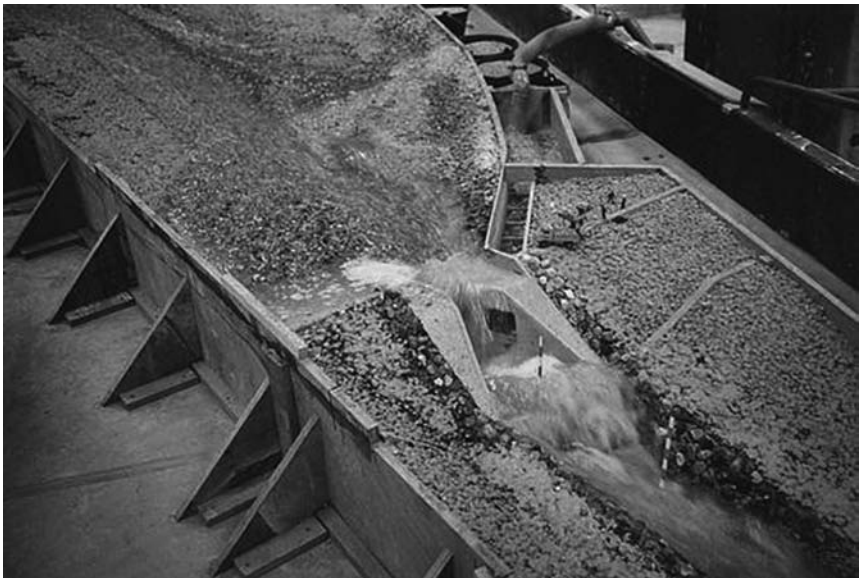
Figure 8.9 The sediment-retaining barrage in the Arve model, M_I = 45 (courtesy of Sogreah, Grenoble)
