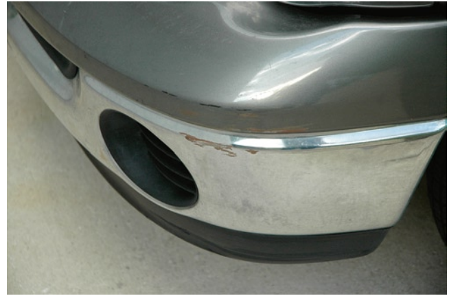
Fig. C.65 Very often, evidence such as this transfer may not be able to be collected in the field. In this case, it has been protected by taping a sheet of paper (a flat bag, sheet of plastic, etc., may suffice) permitting the vehicle to be transported to a secure site accessible to investigators
