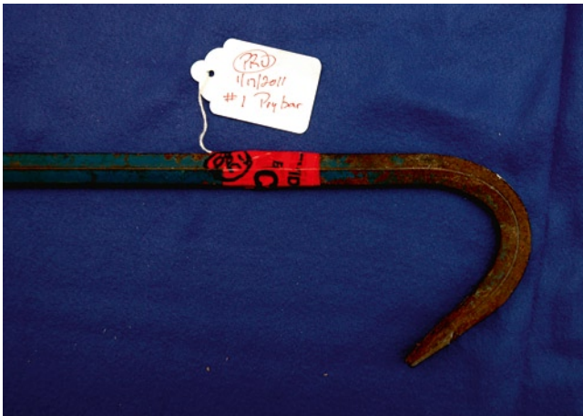
Fig. C.45 String tags are a convenient way to add information to an item that is too large to be conveniently packaged, and which does not require packaging to protect secondary evidence. The tag may be securely attached to the item with appropriate tape
