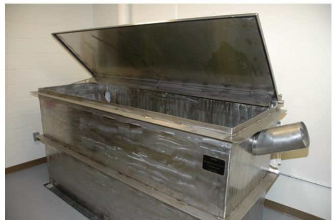
Fig. 3.6 Horizontal shoot tank, designed to permit firing into a pool of water to collect fired projectiles, thus giving the firearms examiner a known standard of the characteristics of a rifled barrel for comparison to an evidence projectile
