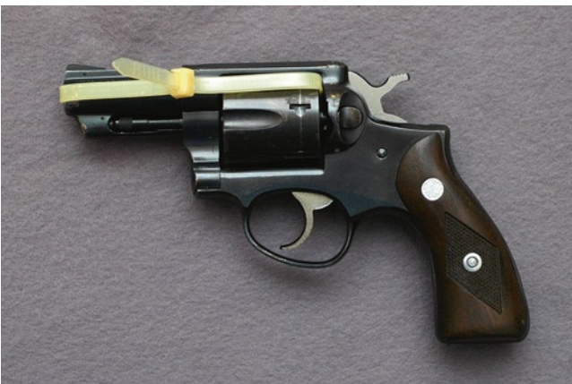
Fig. C.57 The revolver has been made safe by passing a cable tie through the barrel and top chamber, and then locking the tie
