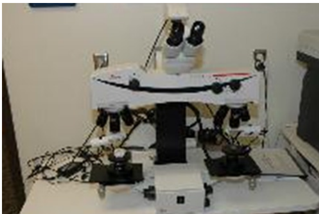
Fig. 3.4 A comparison microscope, the primary tool of the forensic firearms examiner, permitting side by side comparison of the minutiae appearing on known and crime scene evidence
