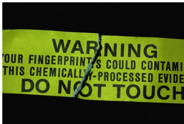
Fig. 3.18 Torn piece of paper tape showing fracture match
