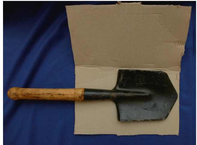
Fig. C.28 These three illustrations show wrapping the blade of a shovel, which may contain trace evidence or may be the source of tool-marks. Depending on circumstances the cardboard may be marked directly or it may be overpacked in a bag
