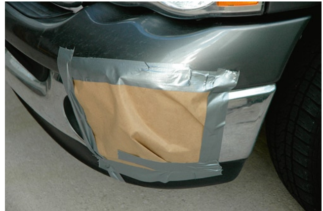
Fig. C.66 Very often, evidence such as this transfer may not be able to be collected in the field. In this case, it has been protected by taping a sheet of paper (a flat bag, sheet of plastic, etc., may suffice) permitting the vehicle to be transported to a secure site accessible to investigators
