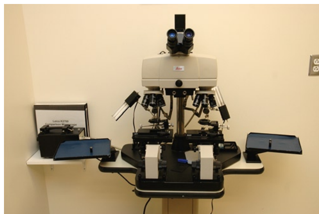
Fig. 3.8 Comparison microscopes are also used in the comparison of know/standard hair and fibers with those recovered on a scene
