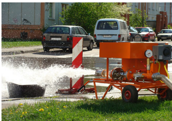
Fig. 15.10 The mobile hand cart with equipment for UDF and RPM procedure in Latvia
