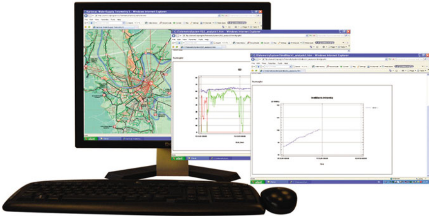
Fig. 13.12 Data web portal of integrated telemetry, AMR/AMI, and system for detection of water leaks and accidental occurrences in water distribution networks
