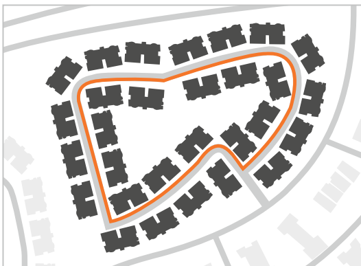
This single-loop road only allows for one path through this development.
