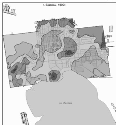
Figure 5. Intensity of the exposition dose of gamma rays of the soil of Balkhash Reference: Gamma rays, A/kg. Range of variation of the isoconcentrate from 10 to 20
