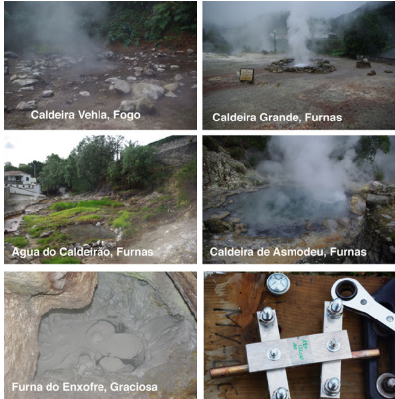
Fig. 2 Some thermal springs in the Azores and the sampling technique of water samples. Copper tubes are clamped in order to collect few grams of water, which will allow the measurement of dissolved helium and neon. Gas can be sampled by accumulation of gas bubbles under a bucket and then collected either in clamped copper tube or reservoir with valves
