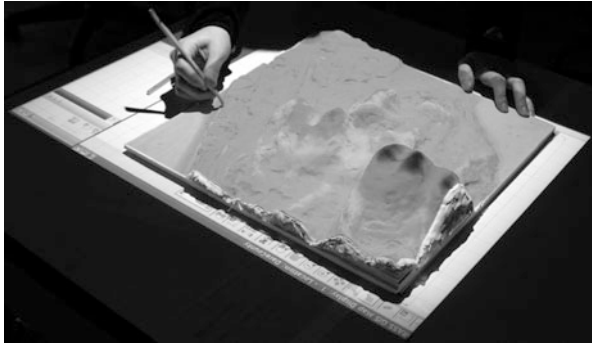
Fig. 2.3 A researcher using the Tangible Geospatial Modeling System [79] to explore the process-form interactions of dune morphology and storms on the Outer Banks of North Carolina
