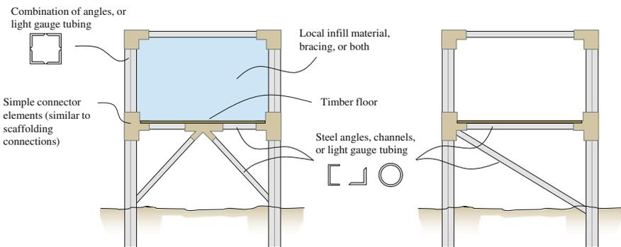
Fig. 19.7 Example multi-purpose element shelter configurations
