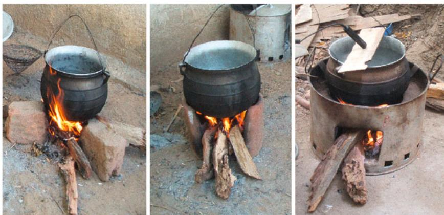
**Fig. 11.1** Different wood stove models tested in the study (3-stone fire, ceramic stove and centrafricain stove)
