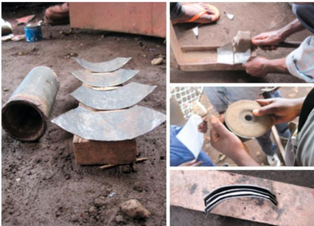
**Fig. 5.5** Blade forming (Ho-Yan 2011d)
