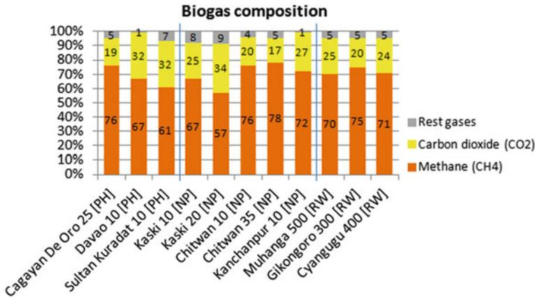
**Fig. 6.5** Comparison of biogas composition in AD systems of Philippines [PH], Nepal [NP] and Rwanda [RW]
