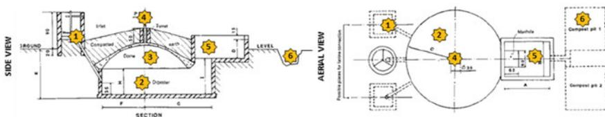
**Fig. 6.1** Side view and aerial view of typical fixed dome underground digester (GGC2047); 1: Inlet chamber with inlet pipe, 2: Digester, 3: Dome (gas storage), 4: Gas outlet, 5: Compensation chamber with overflow point, 6: Storage/compost pit
