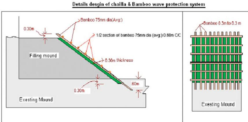
**Fig. 21.4** Design of a *hati* (reprinted here with kind from permission HELVETAS Swiss Intercooperation, Zahid Hasan)
