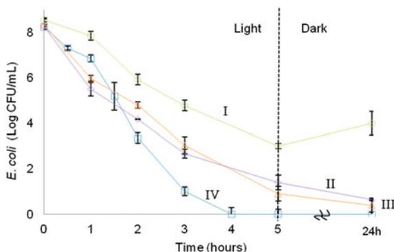
**Fig. 10.2** *E. coli* inactivation (○) simulated solar light (I); (◇)  $Fe^{2+}$  under light (12 mg/L (dissolved iron 3.4 mg/L)) (II); (△)  $Fe^{3+}$  under light (12 mg/L (dissolved iron 2.1 mg/L)) (III); (□) near-neutral photo-Fenton  $Fe^{2+}$  (0.6 mg/L)/ $H_2O_2$  (10 mg/L)/simulated solar light (IV). Simulated solar light intensity ( $520 W/m^2$ ). Experiments were conducted in triplicate and standard error was found to be around 5%
