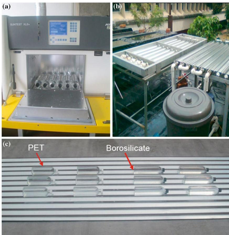
**Fig. 10.1** Different solar water disinfection systems: (a) Solar Simulator (Suntest CPS); (b) CPC reactor exposed to natural sunlight, used at the University of Valle-Colombia; (c) borosilicate and PET bottles placed on an aluminum platform
