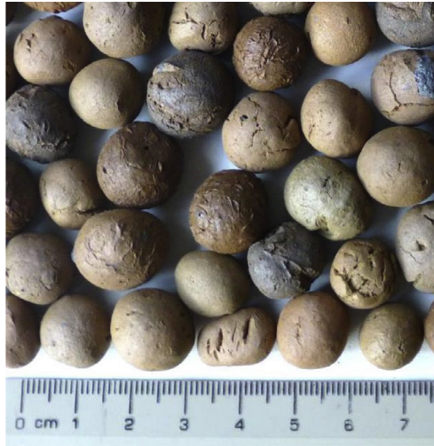
Fig. 10.20 LWA produced in the bench top kiln from London clay ex Crossrail. Particle density: 665 \text{ kg/m}^3 ; 30 min water absorption: 6.8%.
