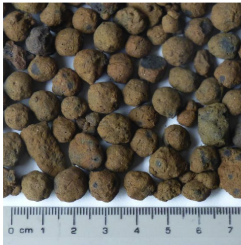
Fig. 10.8 Particle density: 1460 \text{ kg/m}^3 ; 30 min water absorption: 10.5%.
