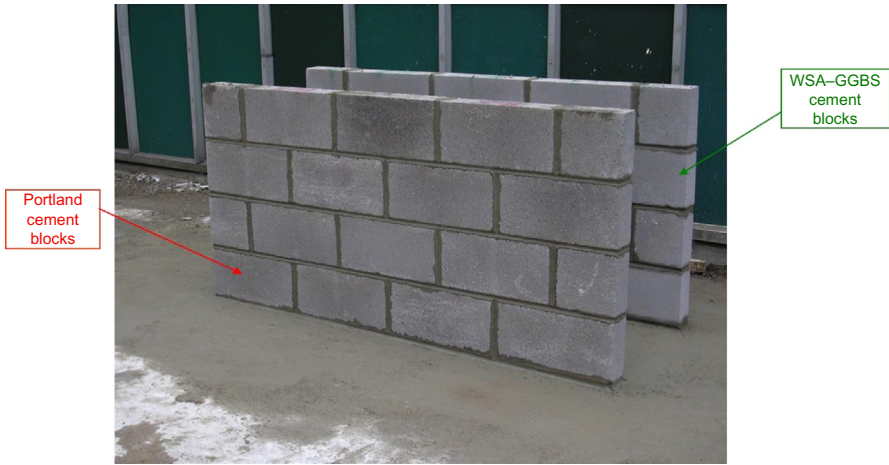
Fig. 22.12 Demonstration of two concrete block walls that showcase the utilization of wastepaper sludge ash (WSA) in the development of ‘green’ cement. Courtesy: Author.
