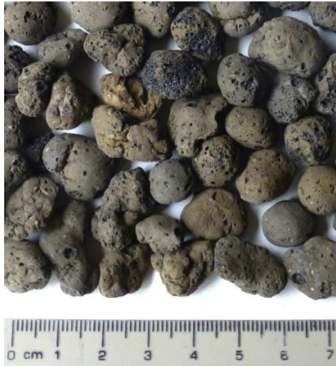
Fig. 10.9 Particle density: 595 \text{ kg/m}^3 ; 30 min water absorption: 18.5%.
