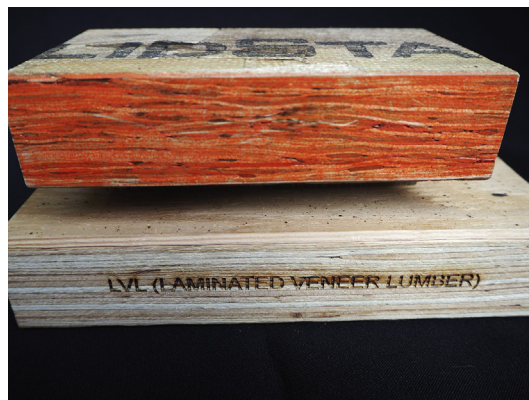
Fig. 8.5 Laminated strand lumber ( top ) and laminated veneer lumber ( bottom ).
