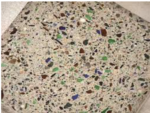
Fig. 5.7 Use of glass aggregate in concrete.
