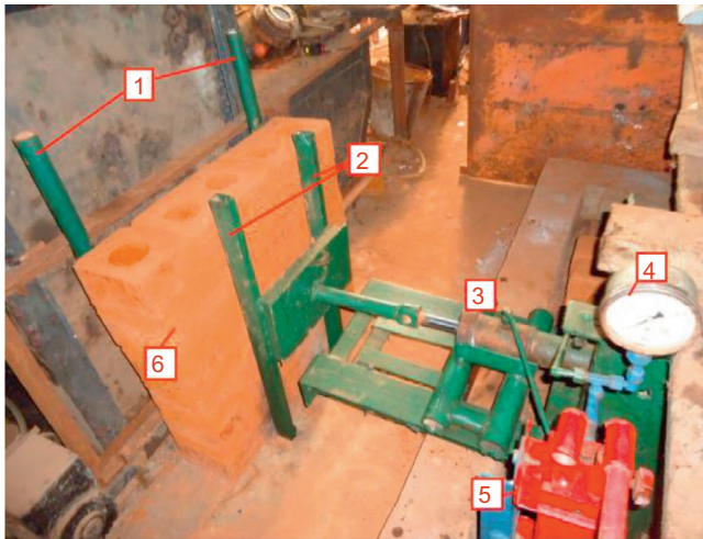
Fig. 13.9 Flexural strength apparatus. 1—Outer bearing; 2—inner bearing; 3—hydraulic press; 4—radial load gauge; 5—hydraulic hand pump; 6—SCEB wall panel or wallette.
