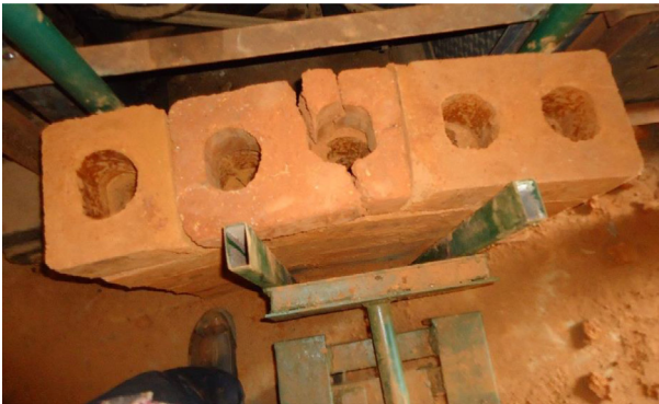
Fig. 13.21 Typical failure pattern of flexural strength test.
