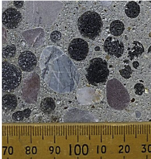
Fig. 10.12 The interior of concrete sawn to expose the coarse aggregate combination of quartzite gravel and Liapor. Concrete density 1925 \text{ kg/m}^3 .
