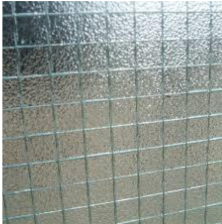
Fig. 5.6 Wire mesh can improve fire resistance, but the surface flaws caused by the wire mesh degrade the strength of the glass.
