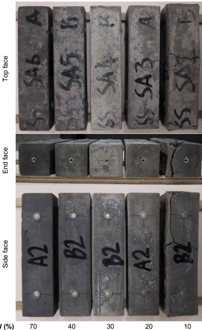
Fig. 26.7 Appearance of C-SDW mortars immersed in sodium sulphate (2.2% \text{Na}_2\text{SO}_4 ) for 365 days.
