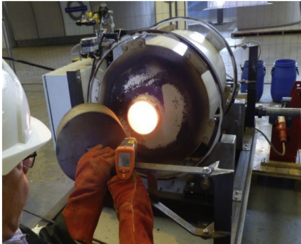
Fig. 10.18 The Sherwin bench top kiln in operation.
