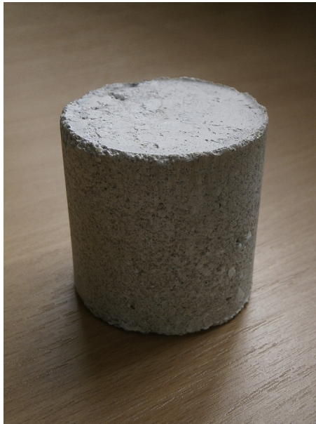
Fig. 25.14 Specimen of phosphogypsum-based concrete with sawdust aggregate.
