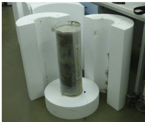
Fig. 10.3 The stripped down insulated mould or pod, showing the concrete encased in the inner acrylic tubular lining, which supported the thermocouples and other instrumentation.
