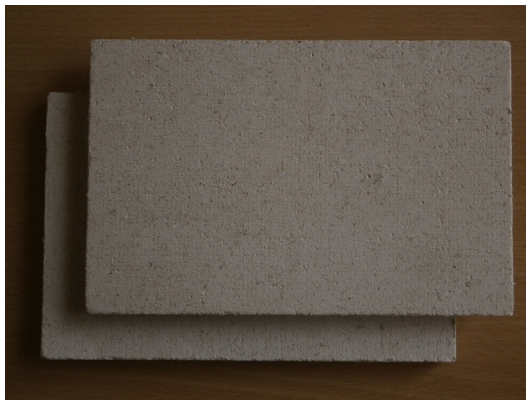
Fig. 25.22 Flooring gypsum fibreboards, thickness 12.5 mm.
