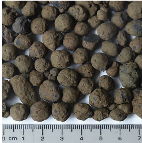
Fig. 10.7 Particle density: 575 \text{ kg/m}^3 ; 30 min water absorption: 13.5%.
