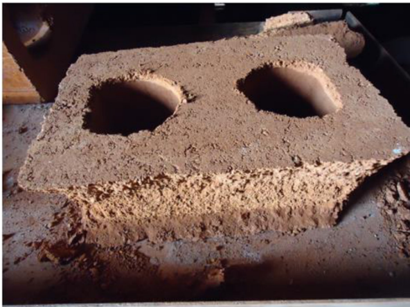
Fig. 13.13 Failure pattern of SCEB.
