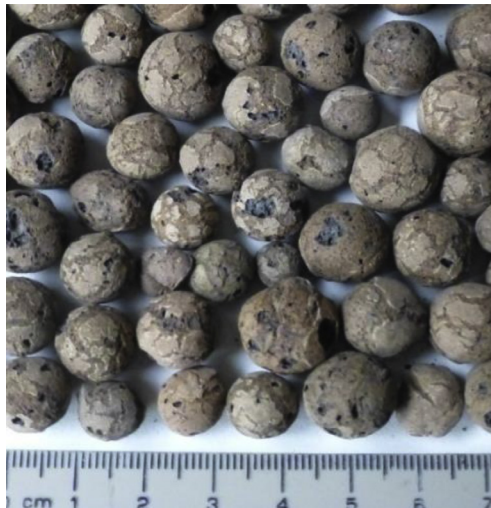
Fig. 10.10 Particle density: 535 \text{ kg/m}^3 ; 30 min water absorption: 21.5%.
