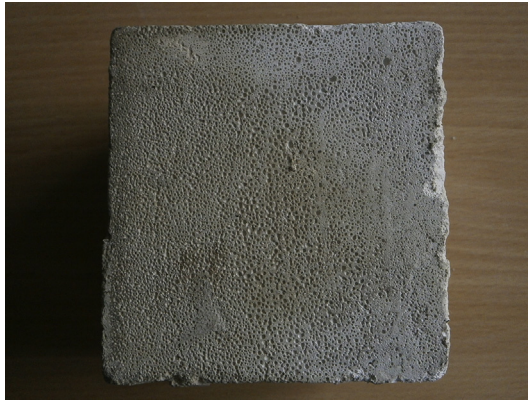
Fig. 25.15 Laboratory specimen of foam gypsum with an average density of 600\text{ kg/m}^3 .
