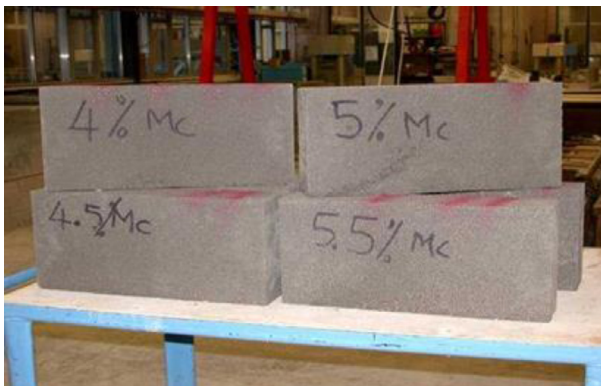
Fig. 22.11 Concrete blocks made with wastepaper sludge ash (WSA; Veerapan et al., 2003).
