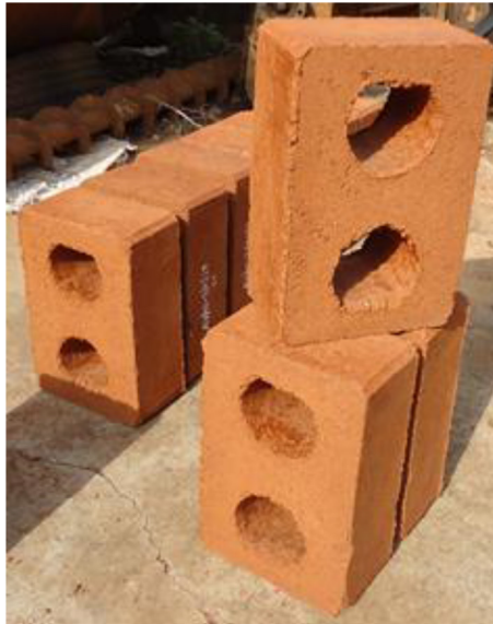
Fig. 13.8 SCEB produced with mechanical kit.
