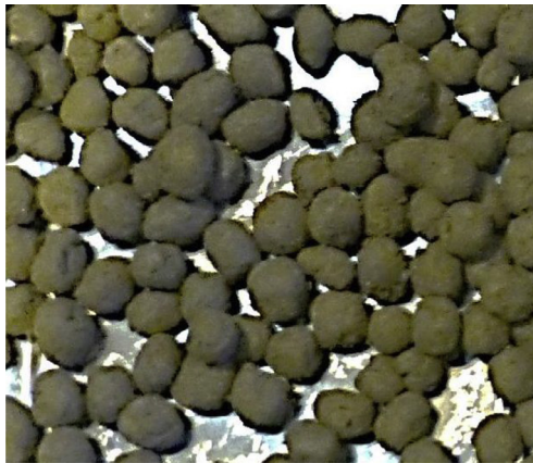
Fig. 10.19 London clay prepared as “green” nodules for firing.
