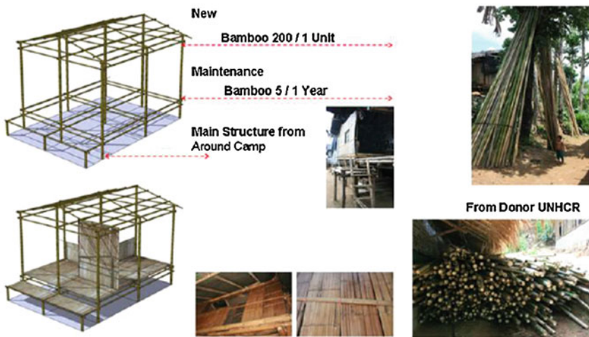
Fig. 4.32 Construction of a one-storey bamboo house. Source Photo taken by study team
