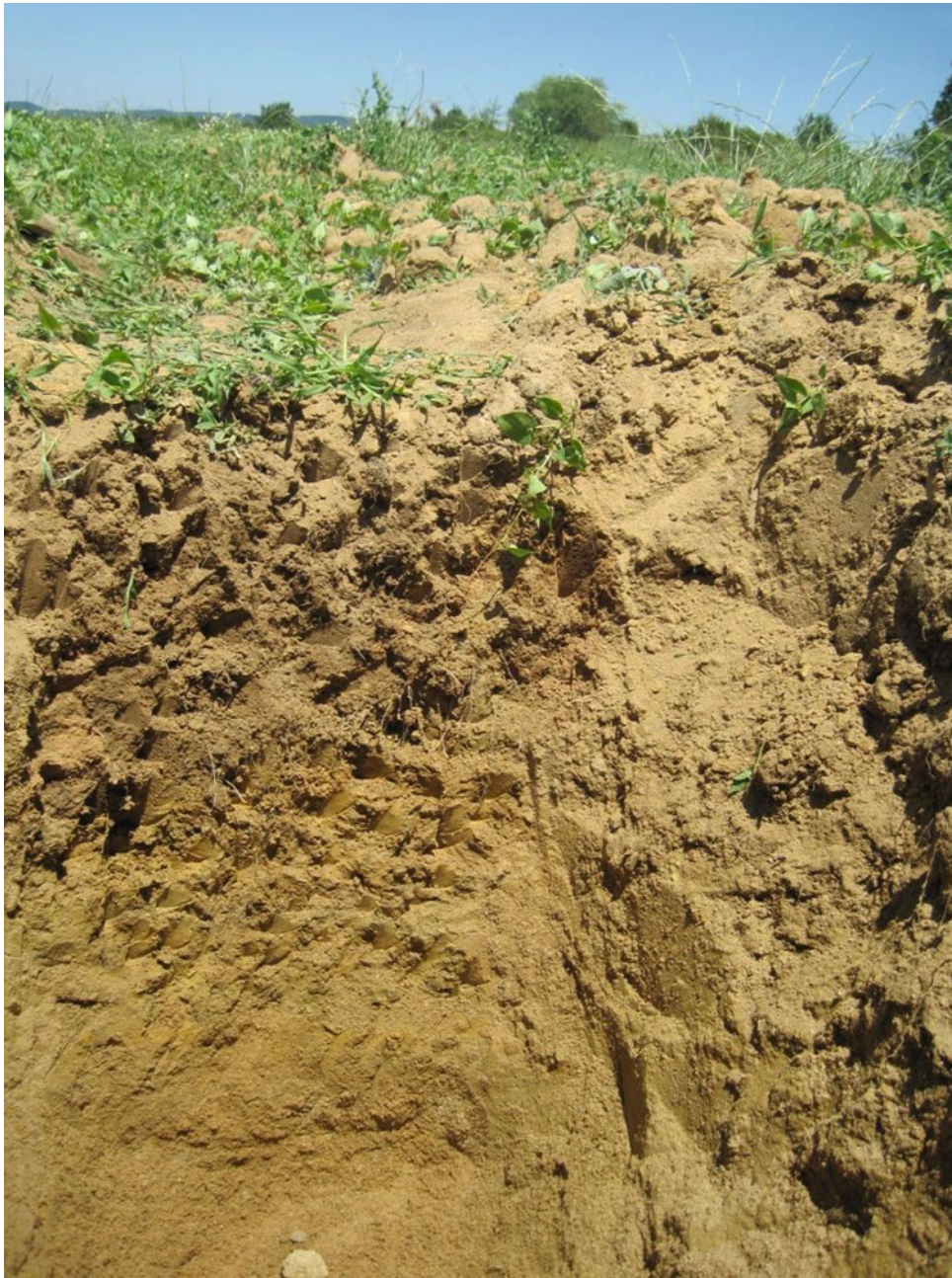
Fig. 13.10 Cinnamonic forest soil severely eroded, Bulgarian classification Yolevski and Hadzhiyanakiev (1976), Haplic Regosol Eutric Siltic , WRB (2006), Typic Xerorthents , Soil Taxonomy (2010), Eutric Regosol , Revised Legend FAO-UNESCO-ISRIC (1990)
