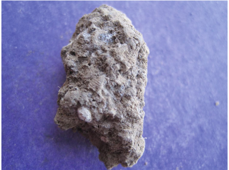
Fig. 2.6 High porous subangular blocky aggregate of B ck horizon saturated with carbonates
