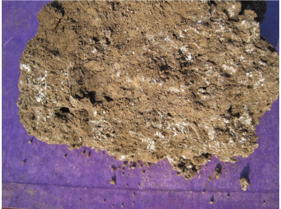
Fig. 2.5 Subangular blocky aggregate with carbonates like pseudomycelium (threads) fine pores, few channels of worms, and worm casts
