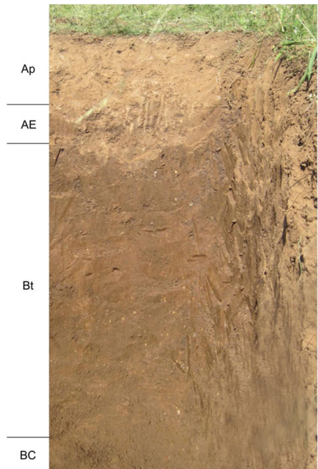
Fig. 7.4 Leached Cinnamonic forest soil, Bulgarian classification Yolevski and Hadzhiyanakiev (1976), Cutanic Luvisol (Chromic) , WRB (2006), Typic Paleustalfs , Keys to Soil Taxonomy (2010), Chromic Luvisol , Revised Legend of the world soils FAO-UNESCO-ISRIC (1990)
