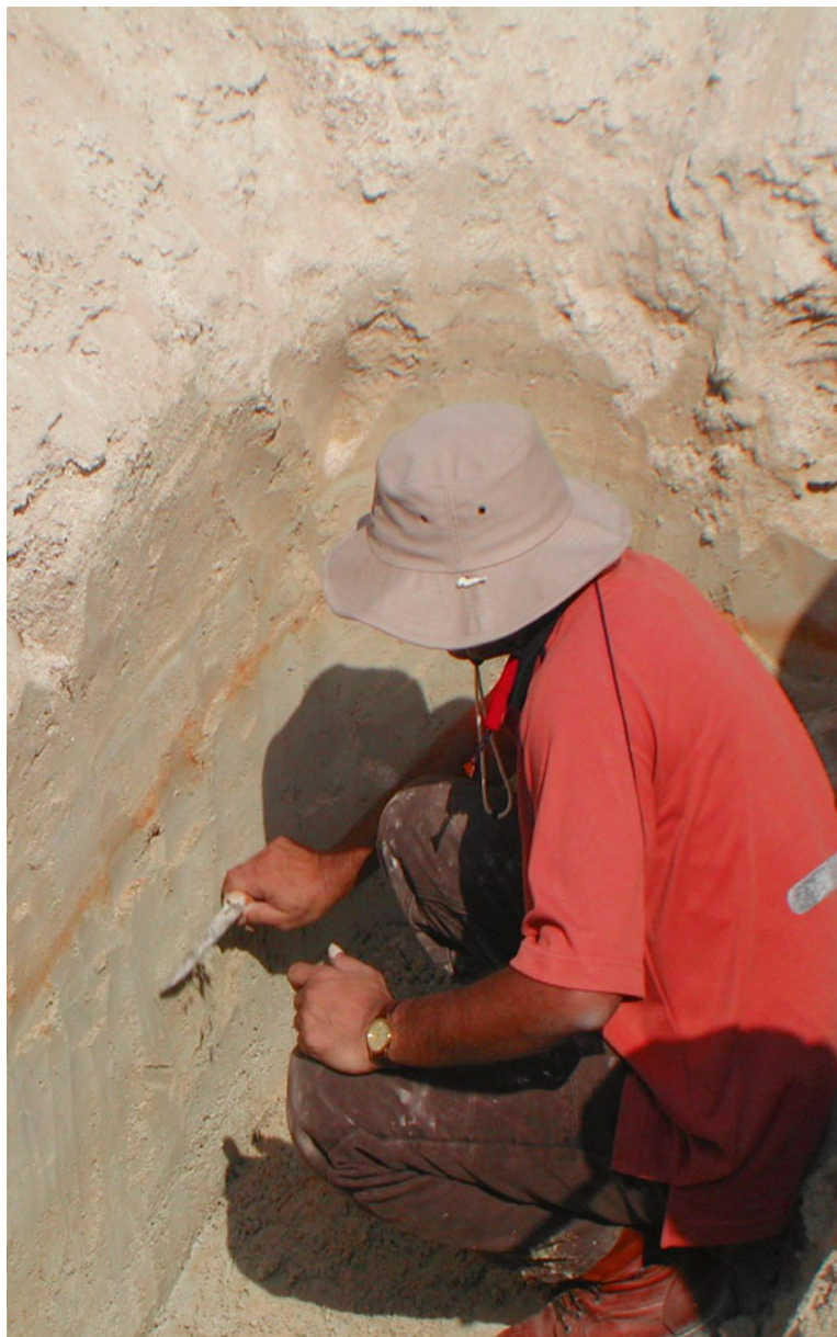
Investigation of the redoximorphic features in a soil from Abu Dhabi coastline
