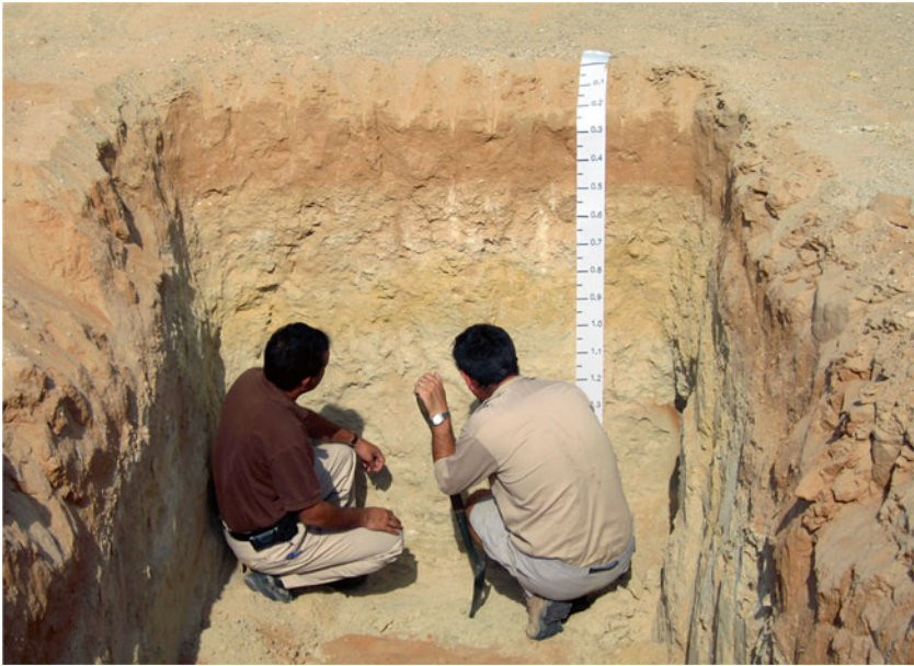
Fig. 2.1 Soil scientists examining and describing a typical soil profile. The scientists document several soil properties and features, commonly to a depth of 2 m. Note the distinct change in horizons (or layers) with depth
