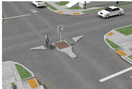
A **channelized right-in/right-out island** forces motor vehicles to turn right while bicyclists can continue straight through the intersection. The island can provide a through bike lane or bicycle access to reduce conflicts with right-turning vehicles.
