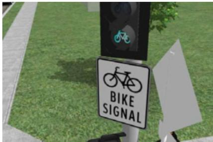
Bicycle signal heads can be added to a hybrid beacon to improve function and safety for bicyclists. See Bicycle Signal Heads for additional guidance.
