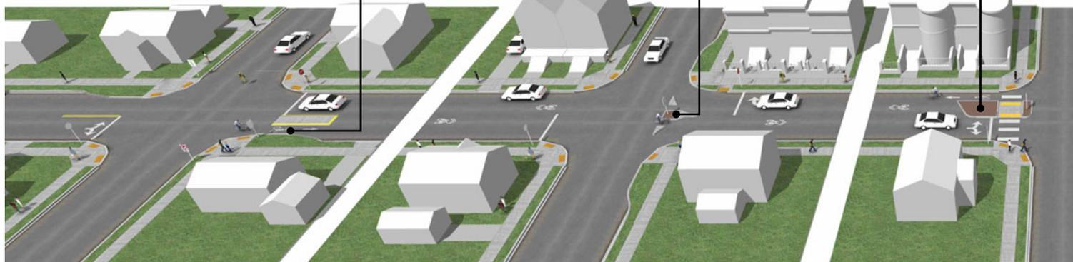
**11** Curb heights lower than 6 inches may be used on diverters and median barriers to allow emergency vehicles to mount and cross barriers.
