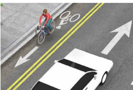
If the connecting street is one way for motor vehicle traffic, consider allowing bicyclists to travel against the flow of traffic using a contra-flow bike lane. **Contra-flow bike lanes** are installed on one side of the street facing one-way vehicle traffic.
