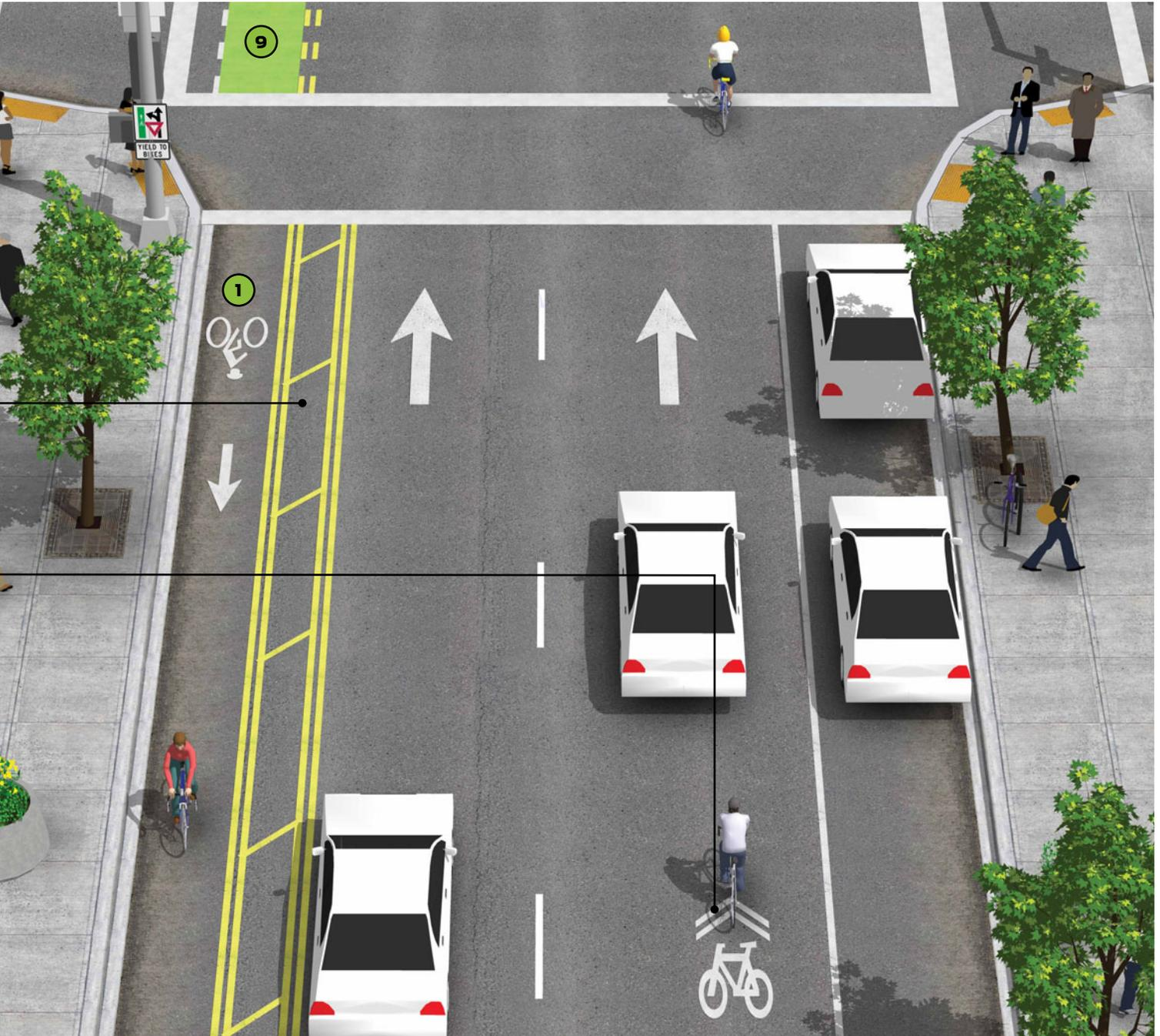
**13** Special consideration should be given before implementing contra-flow bike lanes adjacent to parking. Cars entering and exiting the parking lane will be maneuvering head-on with oncoming bicyclists, introducing an increased speed differential and potentially unfamiliar traffic operations. The driver of a vehicle parked adjacent to a contra-flow lane will have reduced visibility of oncoming bicyclists when compared to parking adjacent to a
