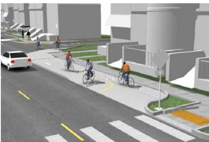
A **two-way cycle track** has the advantage of diverting bicyclists traveling in either direction on a bicycle boulevard to a single crossing location. This minimizes the cost of the crossing treatments and enables the use of beacons and signals, which cannot be used in close proximity.
