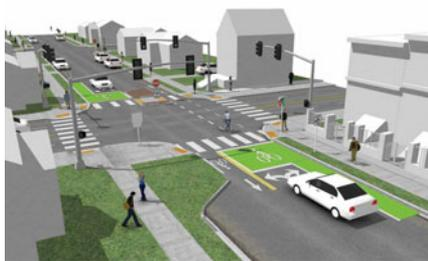
Bike boxes allow bicyclists to get to the head of the queue at signalized intersections. This allows them to take advantage of the typically short green time provided to the minor roadway at an intersection with a major roadway. Such boxes also increase bicyclist visibility to drivers. Parking removal should be considered where a bicycle boulevard has insufficient space to provide the ingress lane to a bike box.
