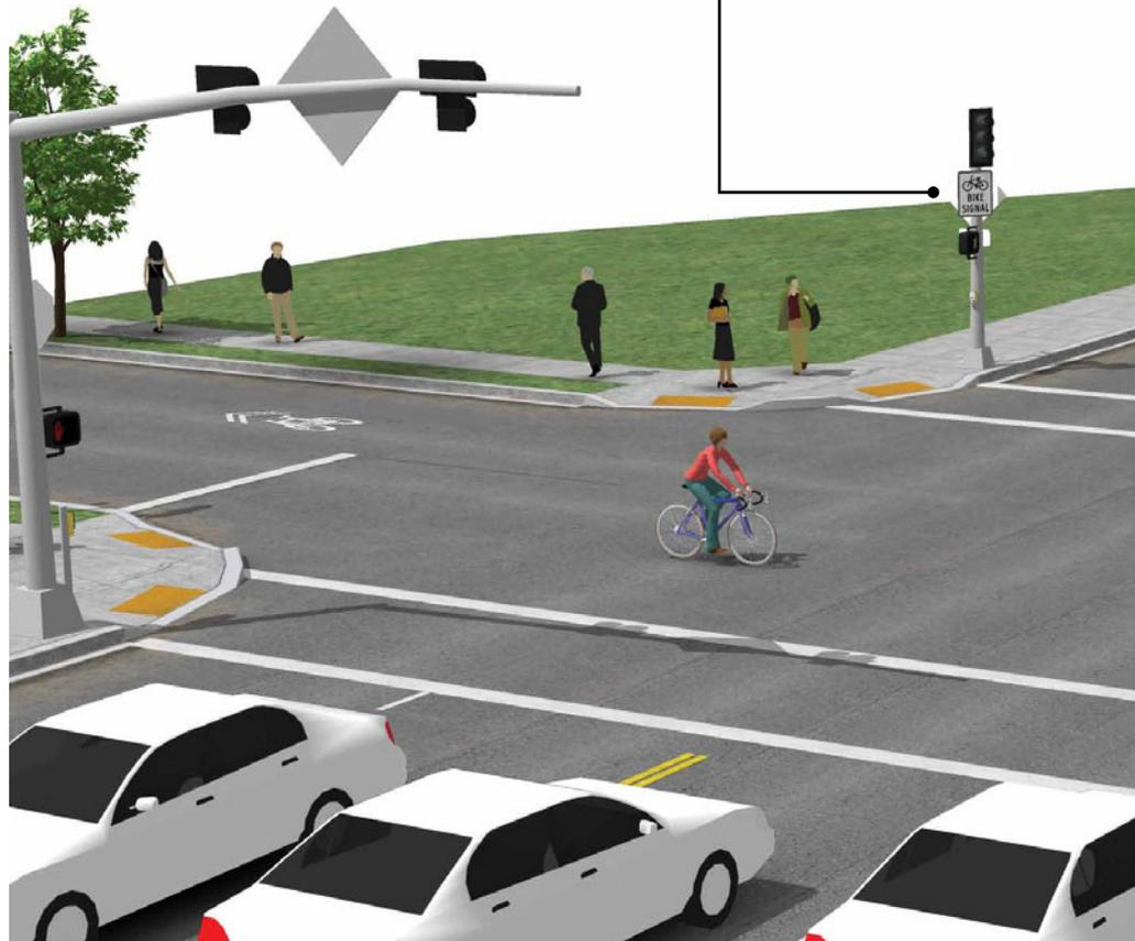
**4** When used to facilitate bicycle movements, a bicycle signal head should be installed in addition to pedestrian signal heads.
