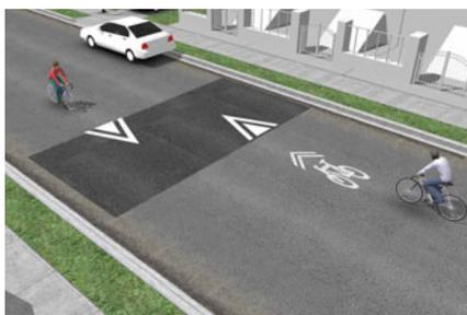
**Speed humps** are 3 to 4 inches high and 12 to 14 feet long, such that speeds are reduced to 15 to 20 mph. They are often referred to as “bumps” on signage and by the general public.<sup>133</sup>
