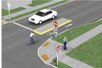
A **forced turn at an intersection** restricts through movements for motor vehicles. This diversion can exclusively use signs to allow buses and emergency vehicles to continue straight, but this may result in poor compliance by motorists (Berkeley, 2000).
