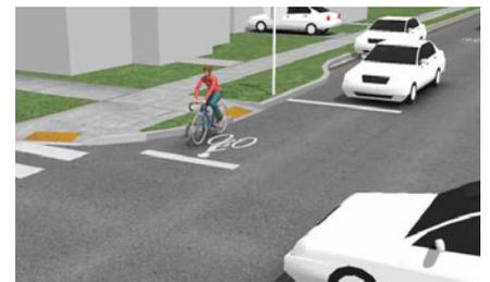
A **bicycle forward stop bar** can reduce the minimum acceptable gap by one second per side of the street.
