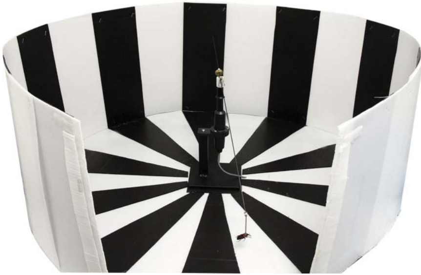
Figure 5.1 Flight mill device in the Volcani Center (Israel) with a tethered red palm weevil at the tip of the rotating arm. Black and white stripes are installed to provide visual stimuli for the flying weevil.
