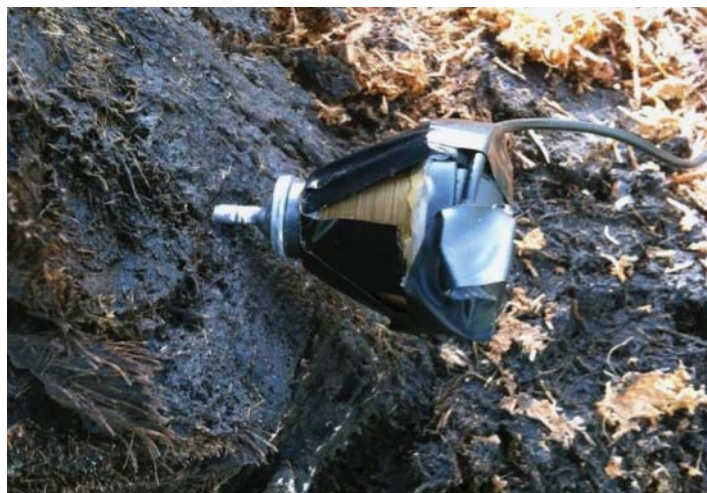
Figure 10.1 Microphone fixed magnetically to a nail inserted into the palm trunk. (Source: Hetzroni 2012)
