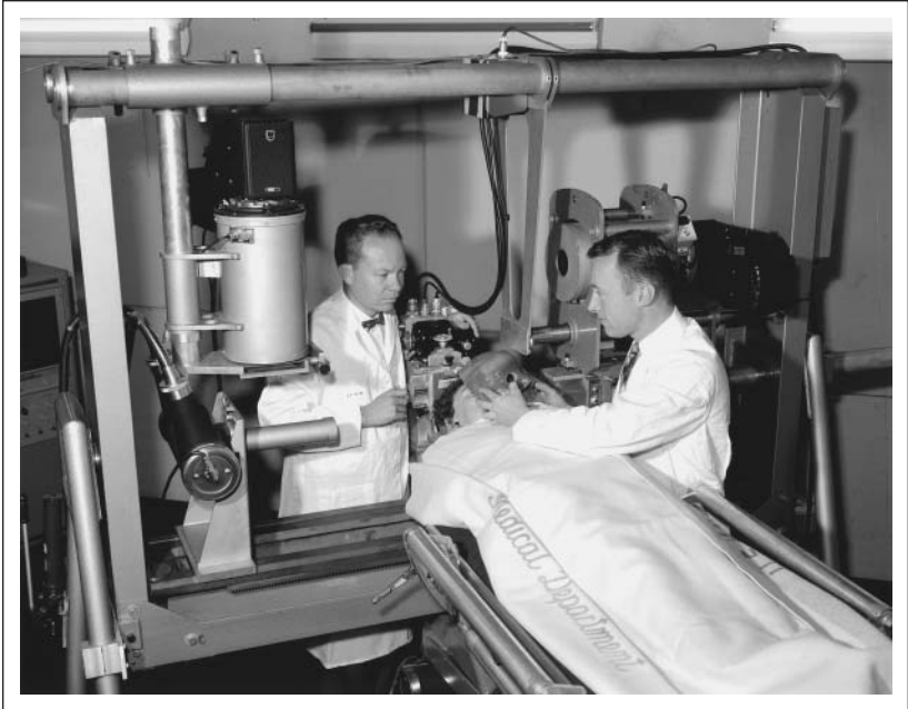
This photo, taken in 1958 at the Lawrence Radiation Laboratory at Berkeley, shows Dr. Richard A. Carlson and Hal O. Anger, an electronics engineer, preparing a patient for irradiation using a 184-inch cyclotron (a particle accelerator). Although the cyclotron enabled physicians to detect tumors, it exposed individuals to unhealthy doses of radiation. (Courtesy of Lawrence Berkeley National Laboratory.)
