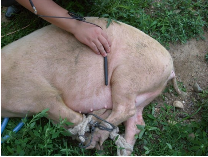
Fig. 4.2 Through-body communication experiment on a pig
