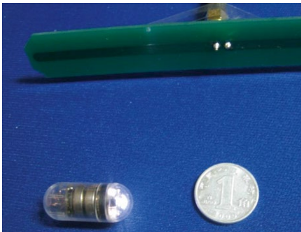
Fig. 5.17 Wireless endoscope capsule switched on wirelessly ( upper : dipole antenna sending switching commands)
