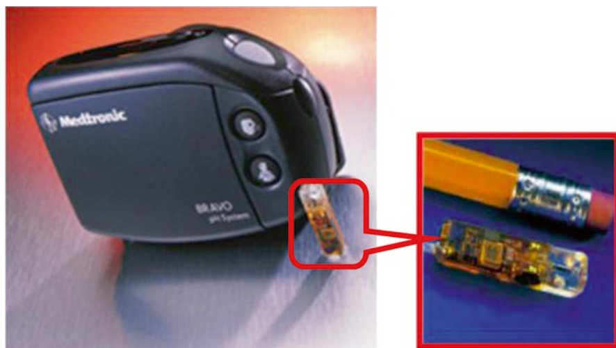
Fig. 3.3 Bravo® pH monitoring system including the pH capsule the portable data receiver, originally manufactured by Medtronic, now acquired by Given Imaging. The pH capsule containing the pH sensor is shown on the right side. The pictures are available online http://www.digestivehealthcare.com/bravo_ph.html
