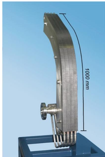
**Fig. 9.7** A water-cooled divertor test surface [31]
