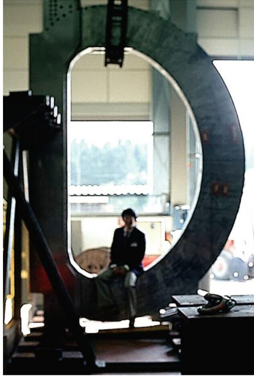
**Fig. 7.12** A D-shaped ASDEX coil
