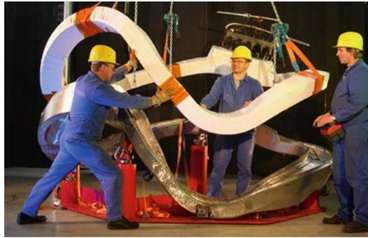
**Fig. 10.4** Two Wendelstein 7-X coils [8]
