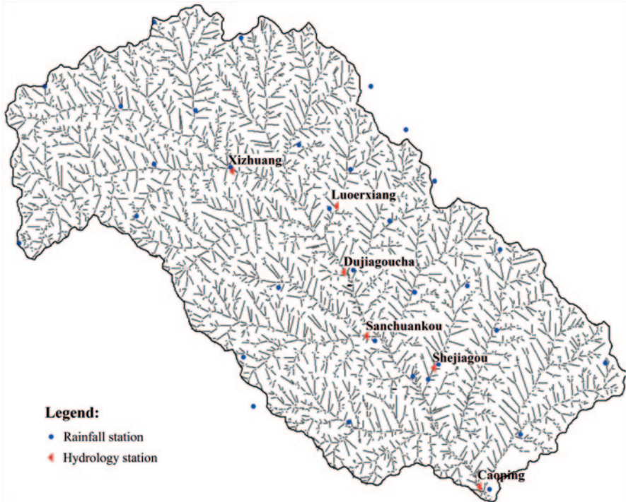
Fig. 1.13 The drainage network of the Chabagou watershed and the distribution of hydrological stations and rainfall stations [16]
