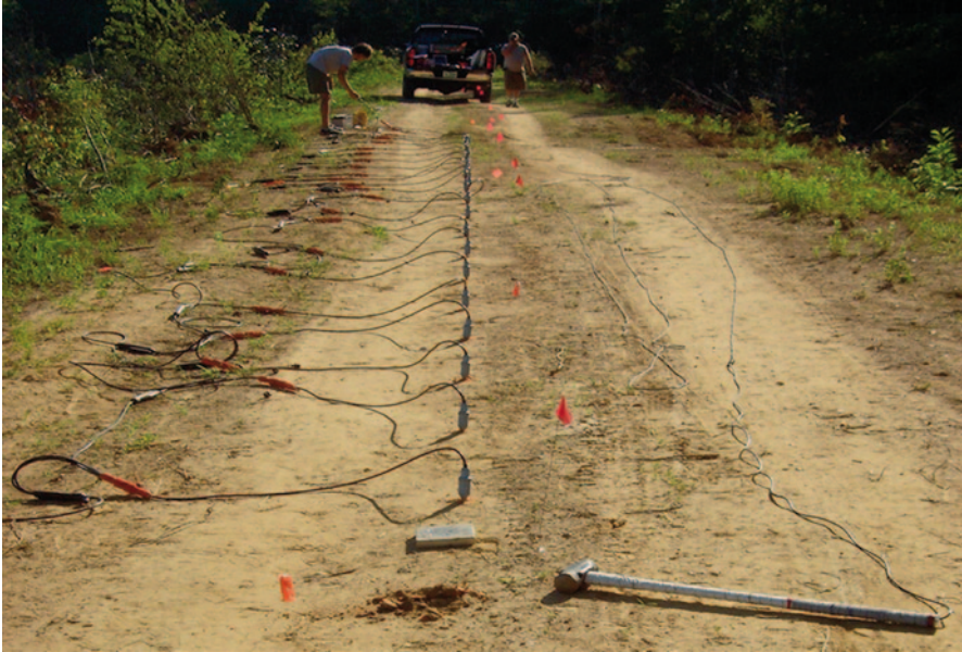
Fig. 7.12 Photograph of a seismic refraction survey on the crest of a dam. A sledgehammer seismic source and a line of 24 geophone receivers are shown
