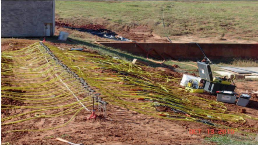
Fig. 7.10 Photograph of an electrical resistivity tomography (ERT) field setup
