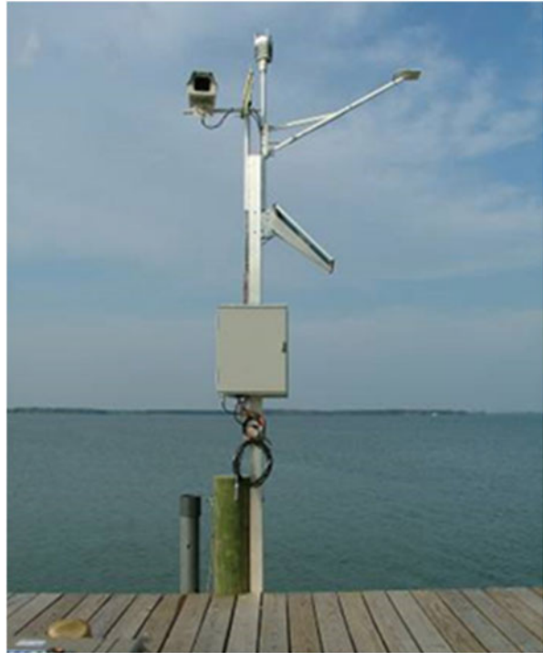
Fig. 18 Example of real-time water quality and water level monitoring, DCPs for Watershed Monitoring. Source: Second author
