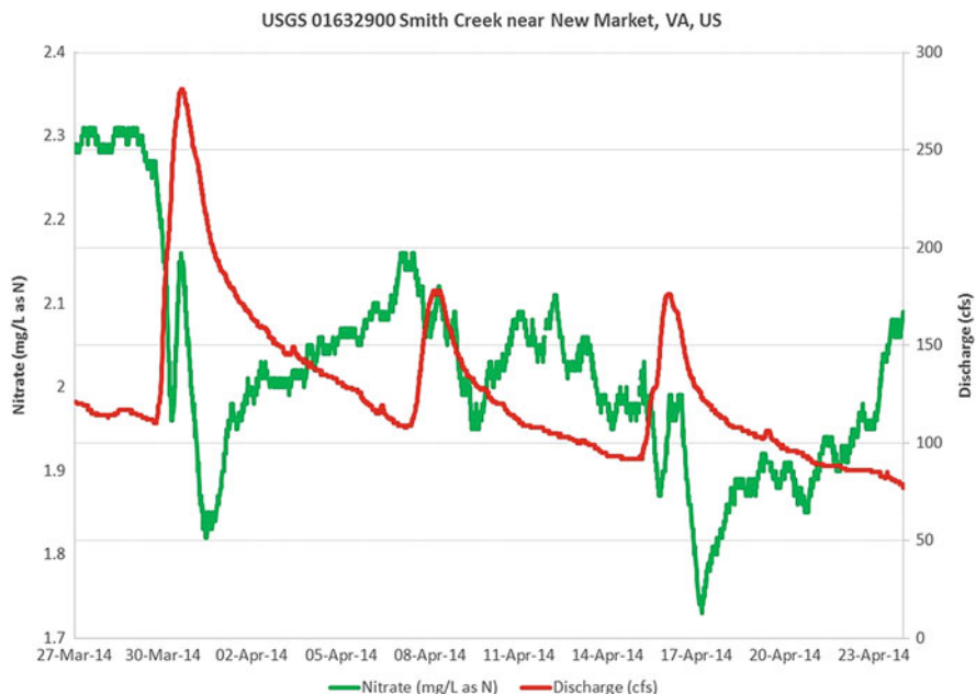
Fig. 14 Real-time nitrate measurements (in mg/L as nitrogen) collected with an optical nitrate sensor and calculated discharge (cubic feet per second) from Smith Creek near New Market, VA, USA (USGS Site 01632900), for the period 27 March–23 April 2014. Source: USGS National Water Information Web Interface. Source: USGS (public domain)
