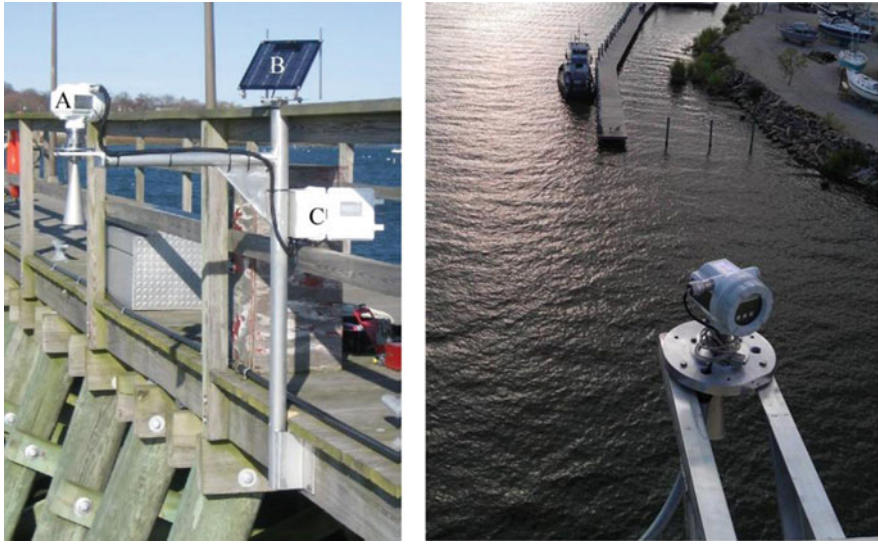
Fig. 4 Tide gauge RADAR-based water level sensor mounted on a pier. Primary components: (A) RADAR sensor, (B) solar panel, (C) data collection platform (DCP). Source: NOAA [3, 4] (public domain)
