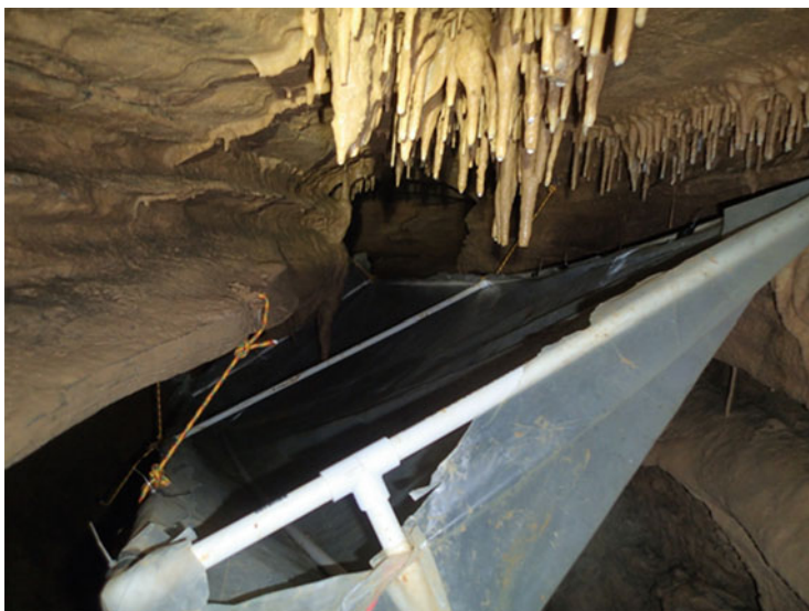
Fig. 6 Tarp system constructed to capture dripwater from speleothems ( Source: Author )
