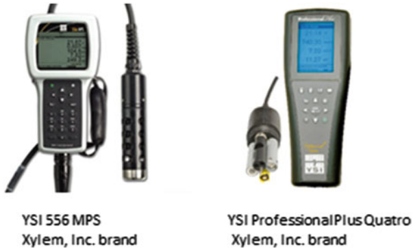
Fig. 15 Examples of handheld water quality instruments for discrete measurements. Source: YSI and Xylem [with permissions from YSI and Xylem]
