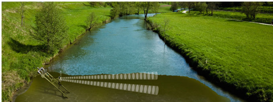
Fig. 9 Illustration of a side-looking ADCP deployed in a small tidal stream with bidirectional flow for continuous measurement of velocity and water level and continuous calculation of discharge. Source: SonTek, a Xylem Inc. (with permissions from Xylem)
