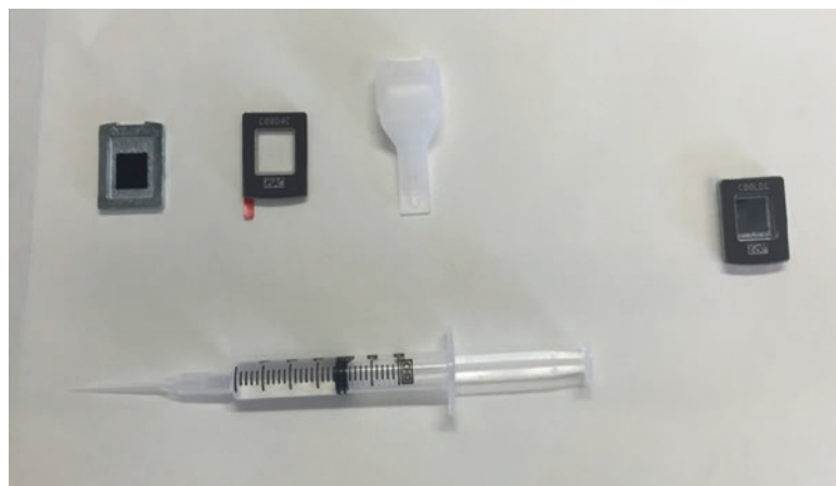
Fig. 2 dPCR kit. Materials provided in the Quantstudio 3D kit for digital PCR (Chip, Chip Lid, Loading blade, and immersion oil syringe). On the right a chip assembled correctly
