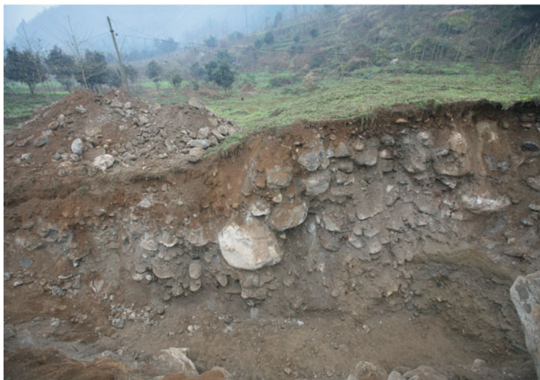
Fig. 4.30 Cross section of the latest surface deformation of fault-related fold scarp developed on the terrace as revealed by the trench on the western side of the highway from Mianzhu to Maoxian at Qingping Village, Mianzhu City. The brown overburden on the bottom of the scarp is thickened, and there is another earlier fold deformation event at the lower part. Viewed to southwest
