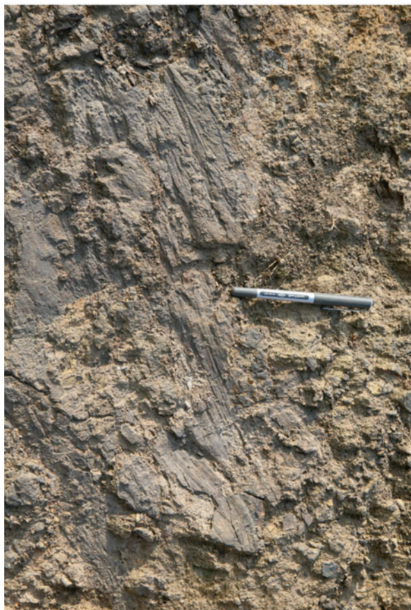
Fig. 4.107 Slickenside striation with a rake variable in the range of 15^{\circ} – 40^{\circ} are developed on the bedrock normal fault plane on the eastern bank of a river near Sujiayuan Village, to the north of Shikan Township, Pingwu County; this may indicate the existence of relatively large right-slip component. Viewed to north
