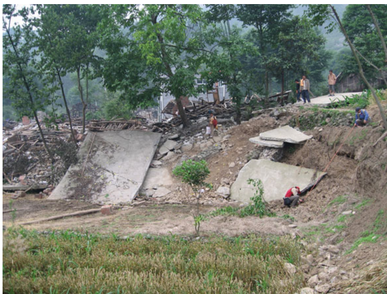
Fig. 4.48 The T2 terrace and the cement road on it was offset by the earthquake fault to form a 2~3 m-high simple pressure ridge in the north of the 1st Group of Shiyan Village, Leigu Town, Beichuan County. The houses on the hanging wall near the fault were completely destroyed, and the trees incline toward the foot wall. Viewed to southeast
