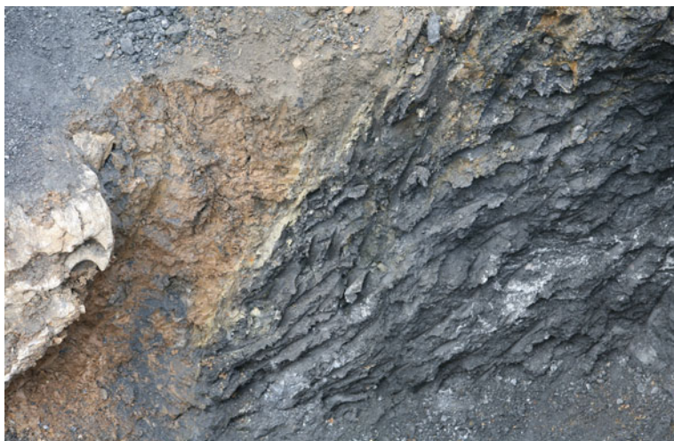
Fig. 4.67 A NW-trending trench excavated across the eastern step-like normal fault scarp on the loess platform at Heshangping Village. The trench reveals the grayish yellow fault gouge materials developed on the newest fault plane between the dark grey broken mudstone and yellowish brown stone-bearing soil bed. Viewed to southwest
