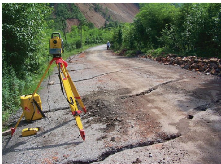
Fig. 4.36 Simple pressure ridge about 2.2 m high and tension crack zone about 180 m wide at Quanshui Village, Gaochuan Township, Mianzhu City. Viewed to southwest
