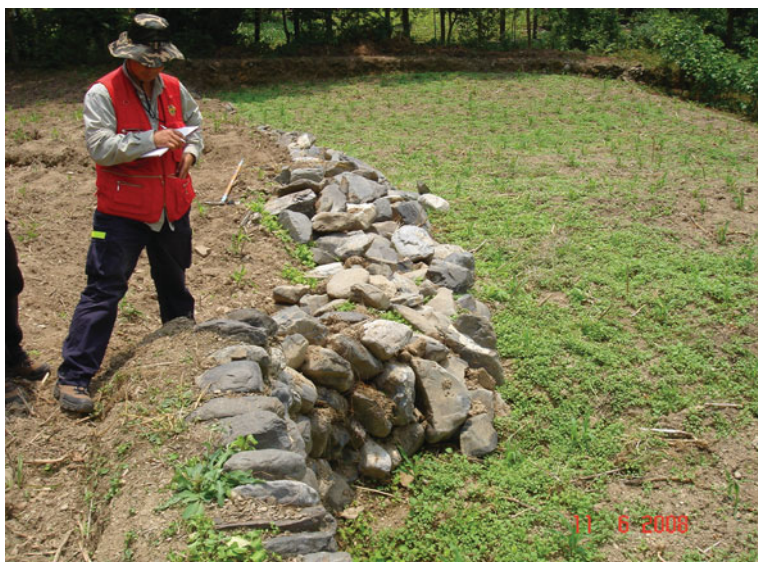
Fig. 4.76 The earth bank between field was right-laterally offset for 1.6 m on the T1 terrace at Fenghuang Village, Guixi Township, Beichuan County. Viewed to southeast
