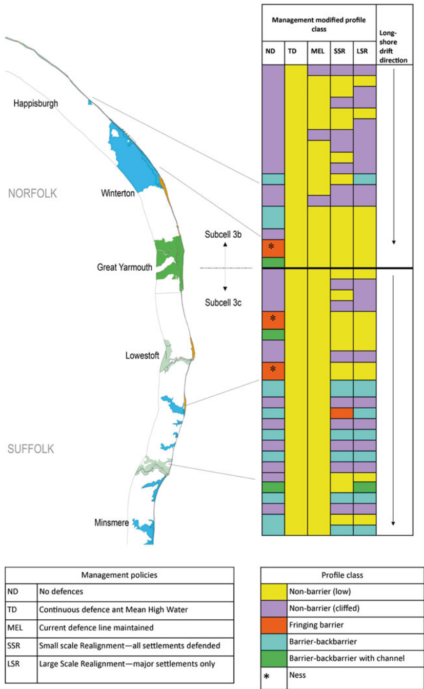
Fig. 5.4 Illustrative section of the East Anglian (sediment subcells b and c ) coast showing the change in the active coastal configuration under the five management options
