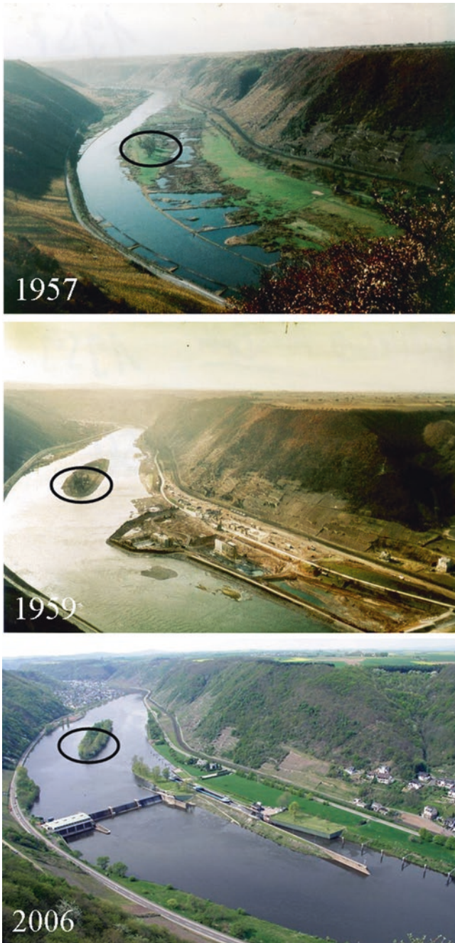
Fig. 14.1 Development of the river Mosel at Lehmen (near the city of Koblenz) from 1957 to 2006 (source Waterway and Shipping Office Koblenz). The black circles show the development of the isle “Reiherschuss” due to the construction of the barrage
