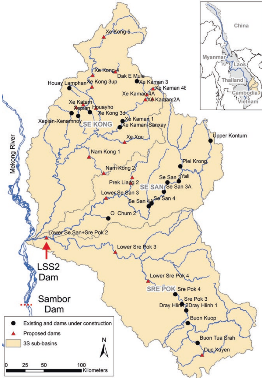
Fig. 2.1 Se San, Sre Pok, and Se Kong (3S) tributary basins to the Mekong River, showing current and future reservoir locations. The red arrow indicates the proposed location of the Lower Se San 2 (LSS2) Dam site, whereas the red dashed line indicates the proposed location of Sambor Dam on the mainstream Mekong River. Modified from Wild and Loucks (2014a).
