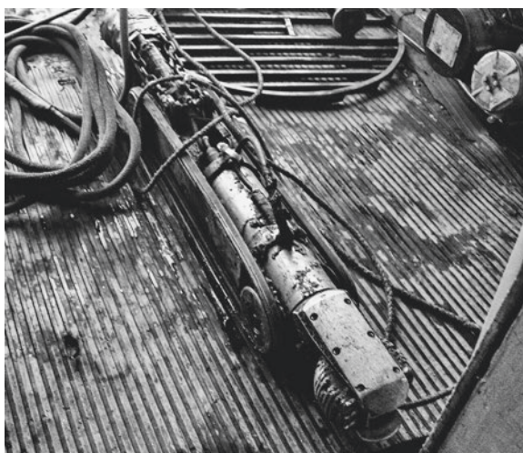
Fig. 10.1 Inspections are typically carried out using robots equipped with cameras that are inserted into a pipe and remotely operated from the road surface
