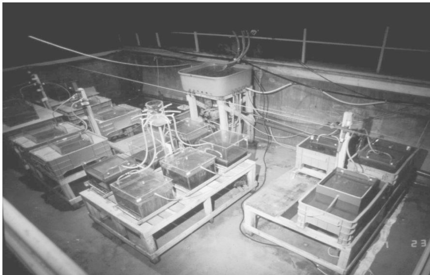
Figure 3: Experimental work with contaminated sediments to measure fluxes of metals from sediments to water.
