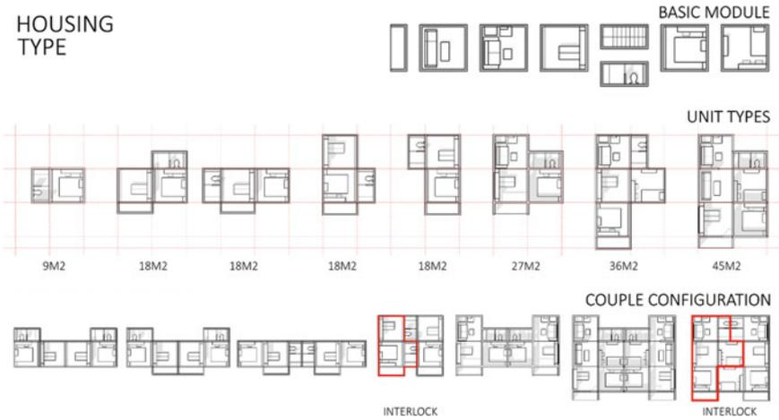
Fig. 12 Housing type modular system. (Source Author)
