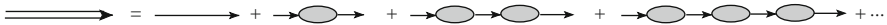
Fig. 26.12. Graphic representation of the full GF as sum of diagrams with free propagators and (irreducible) self-energies. The double line indicates G , simple line G_o , shaded area \Sigma
