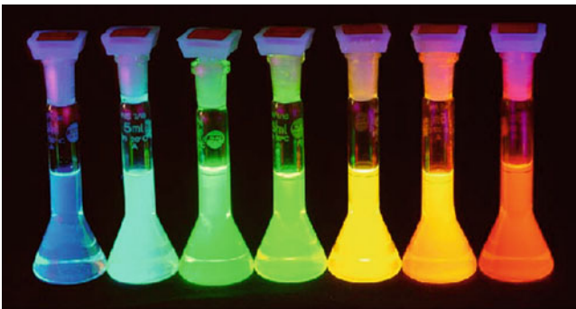
Fig. 22.16. CdSe quantum-dot particles in suspension. Dots of different sizes contain electron states with different energy levels and emit light of different colors (Printing by permission, copyright Prof. H. Weller, University of Hamburg, Germany)
