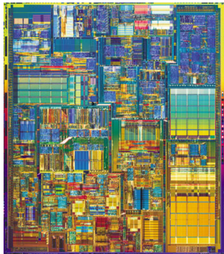
Fig. 22.7. Left: the Intel 4004 microprocessor was the first commercially available microprocessor released by Intel in 1971. It contained 2300 transistors on an area of 13.4 \text{ mm}^2 . Right: the first release of the Pentium 4 microprocessor, available in 2000. This microprocessor contained more than 41 million transistors on an area of 217 \text{ mm}^2 . Nowadays microprocessors have almost one billion transistors on a single chip (Images by courtesy of Intel Corporation)
