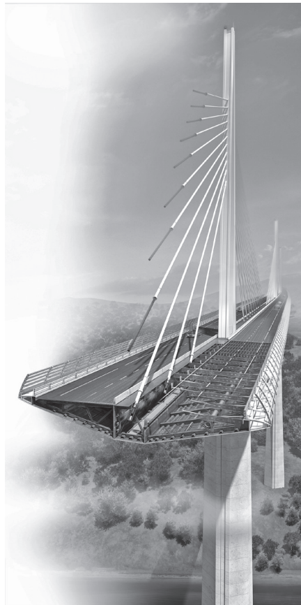
FIGURE 4.7 Cross section of bridge deck. (Architectural drawings provided by Foster + Partners. Image courtesy of Foster + Partners.)
