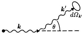
Fig. 3.41. The outgoing photon ( k' ) is scattered with respect to the incoming one ( k ) by an angle \theta into the spherical angle element d\Omega_{k'}
