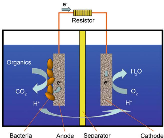
**Fig. 2** Schematic diagram of a typical two-chamber MFC
