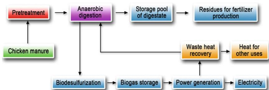
Fig. 2 Schematic diagram of the Deqingyuan biogas power project
