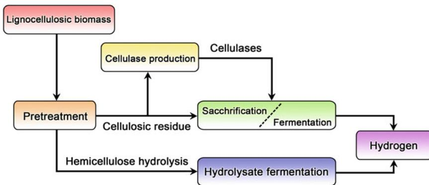
**Fig. 1** General scheme for converting lignocellulosic wastes into hydrogen
