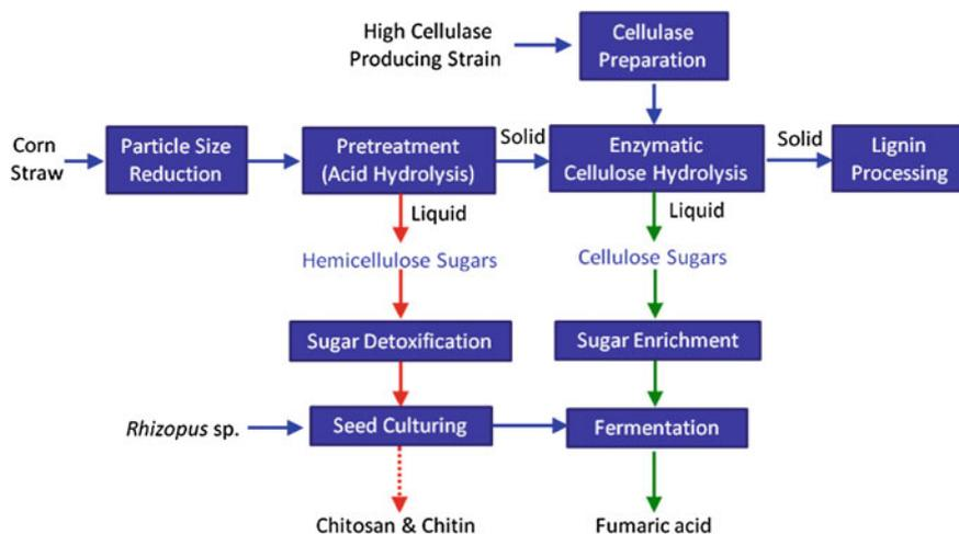
**Fig. 5** Two-stage utilization of the hemicellulose and cellulose components of corn straw for fumaric acid production
