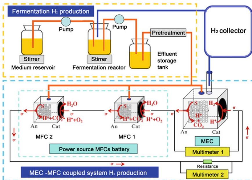
**Fig. 2** Process diagram of the integrated hydrogen production, microbial electrolysis cell (MEC), and microbial fuel cells (MFCs)
