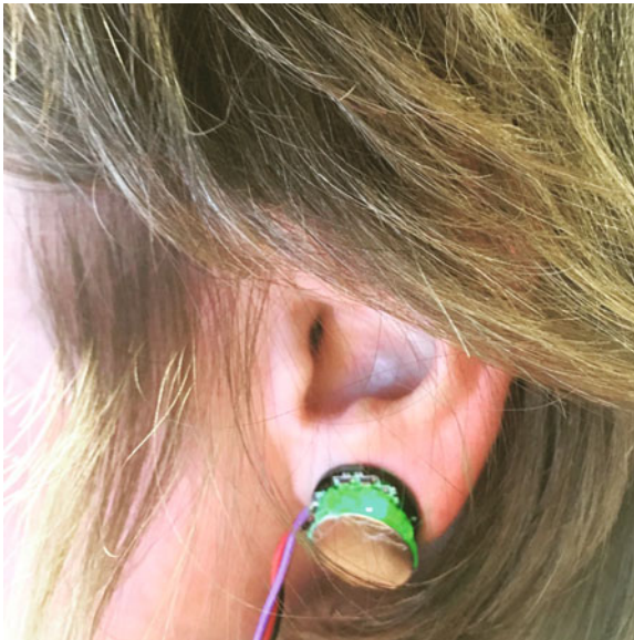
Figure 5-9. IOTPulse Sensor on Ear
