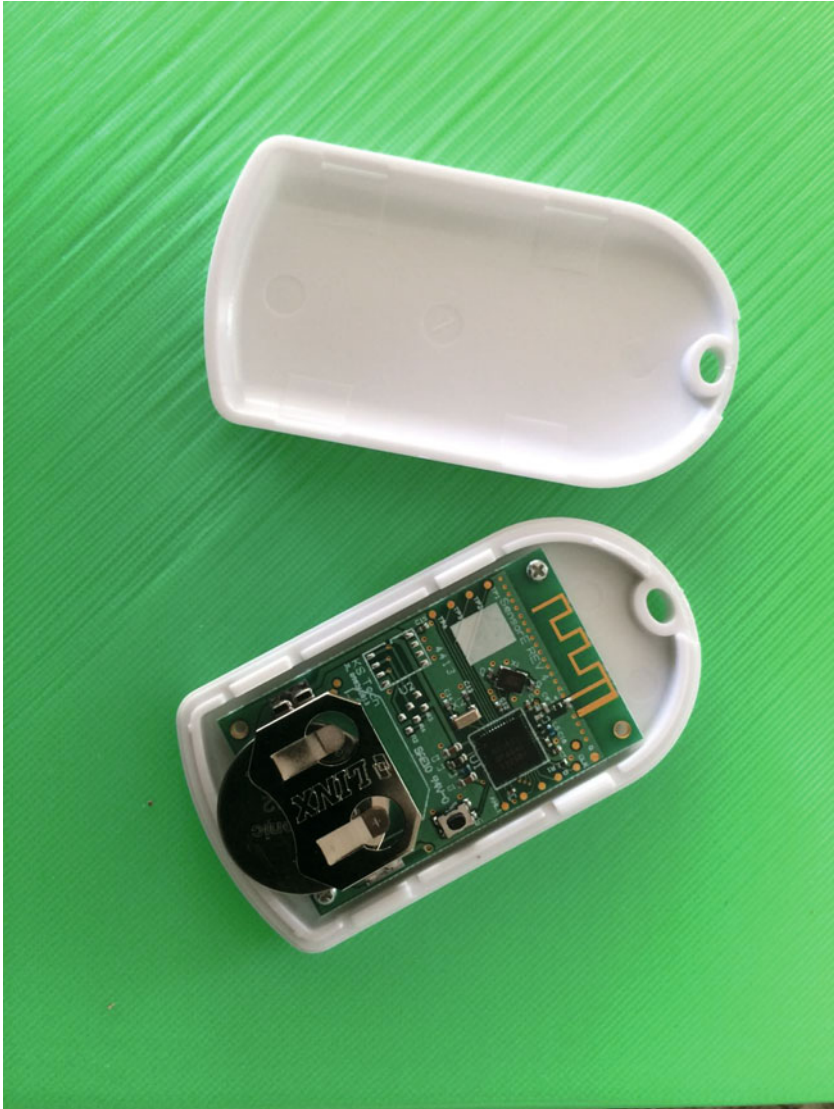
Figure 4-3. Inside of a Particle iBeacon
