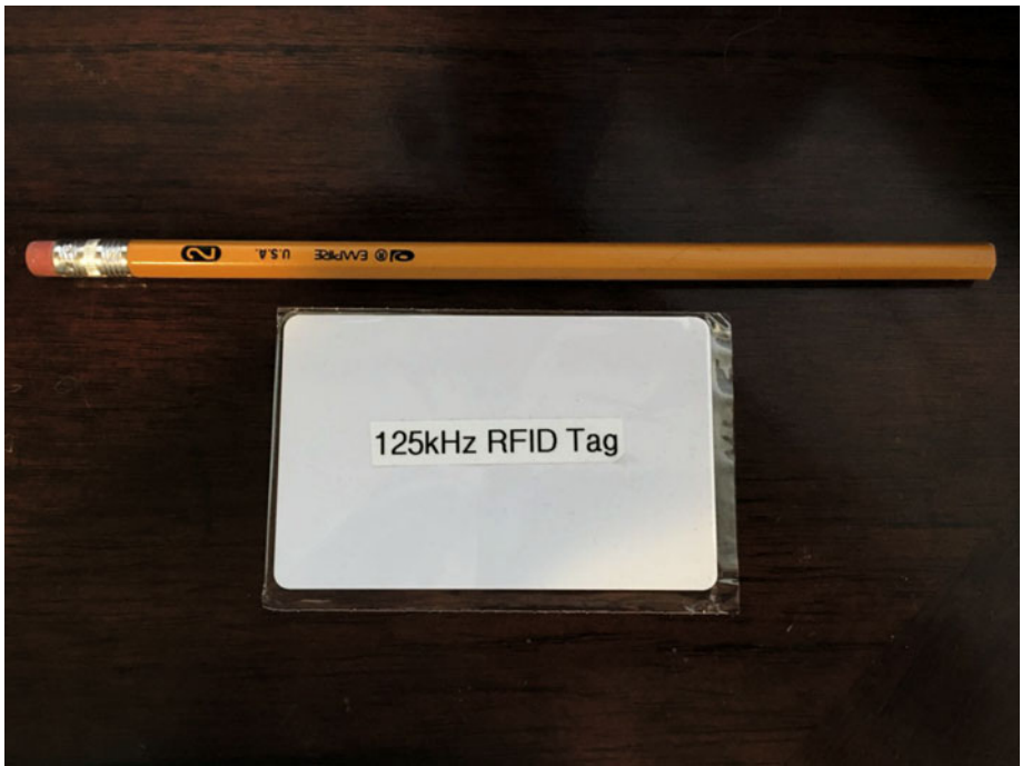
Figure 6-1. 125kHz Card-Shaped RFID Tag
