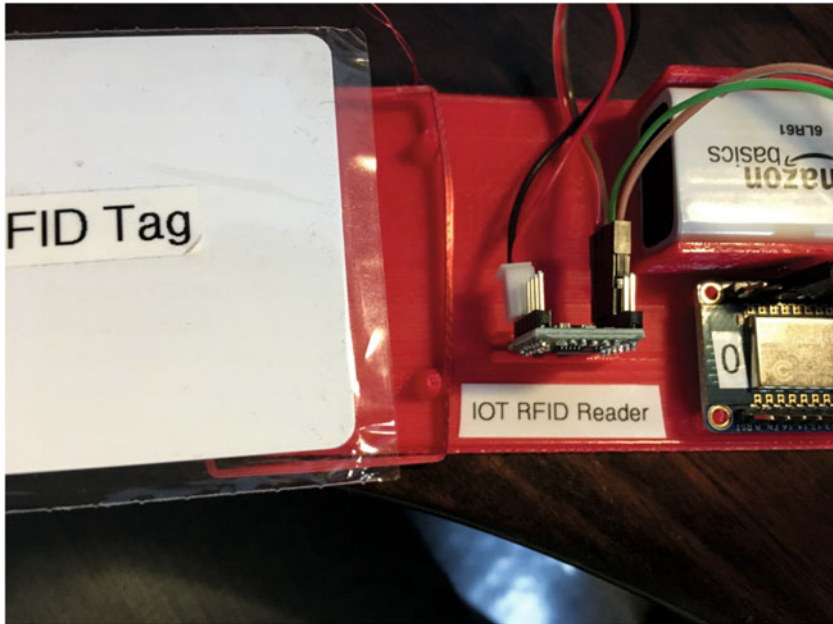
Figure 6-8. RFID Tag Card over the IOTRFID Device
