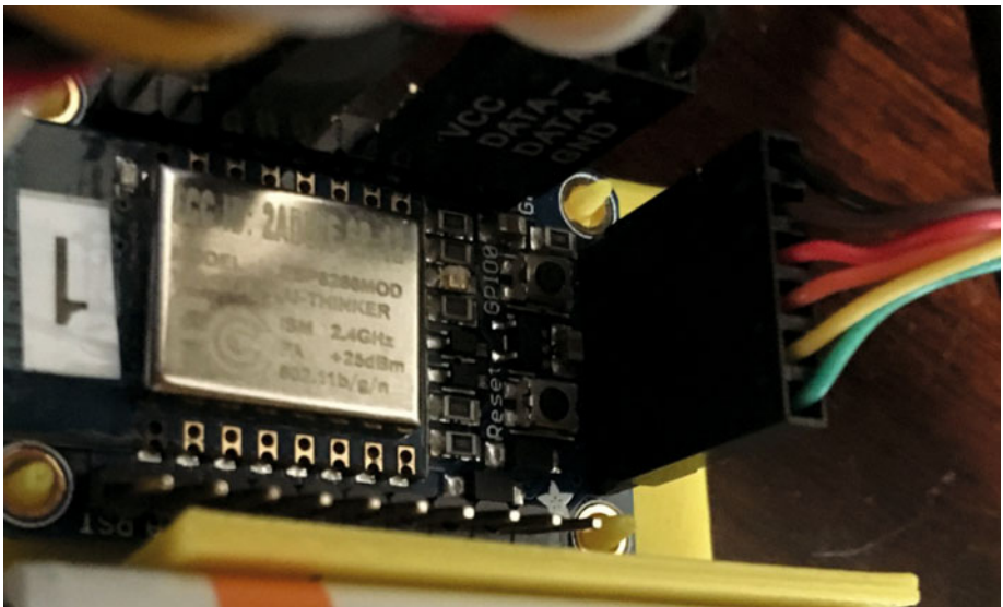
Figure 2-9. FTDI Cable Plugged into ESP8266
