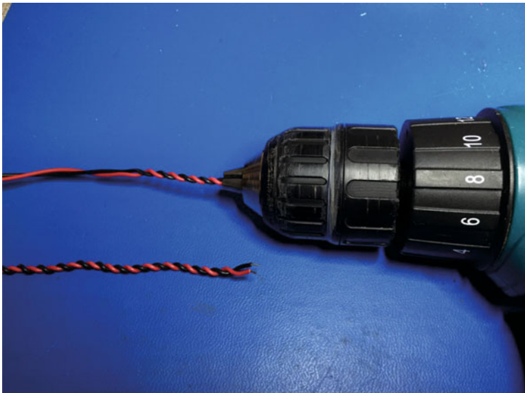
Figure 3-16. Braided Cables with Drill
