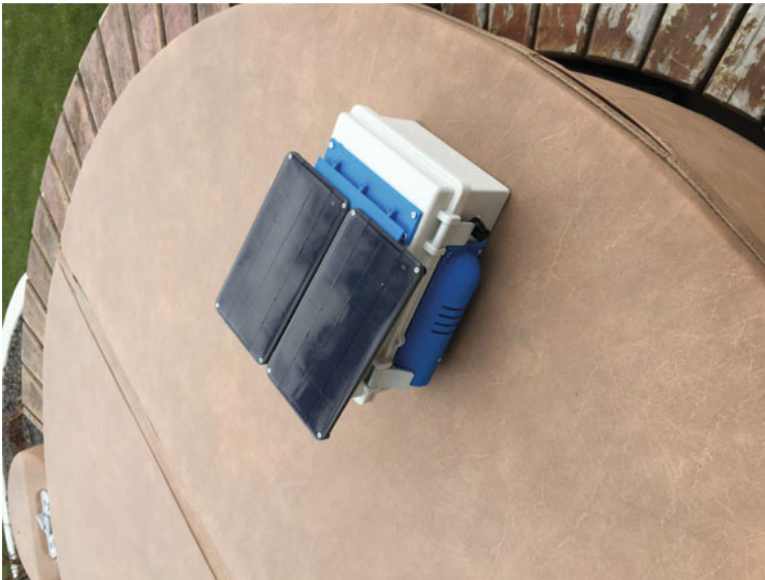
Figure 3-10. Solar Power Panels on IOTWeatherPi
