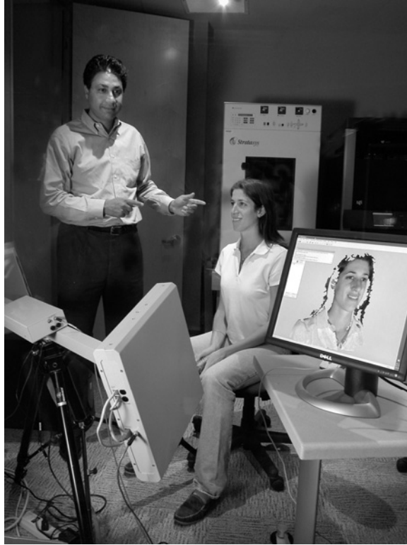
Fig. 1. A multicamera-based 3D face scanner used at the PRISM lab at ASU. The scanned data included both 3D and 2D image. Note the missing data corresponding to the hair of the subject.
