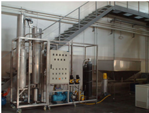
Fig. 13 Pilot plant for the recycling of polystyrene wastes by dissolution at ambient conditions and solvent recovery by scCO 2
