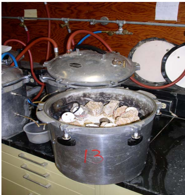
Fig. 2. Pressure-plate extraction at 33-kPa for clods.
