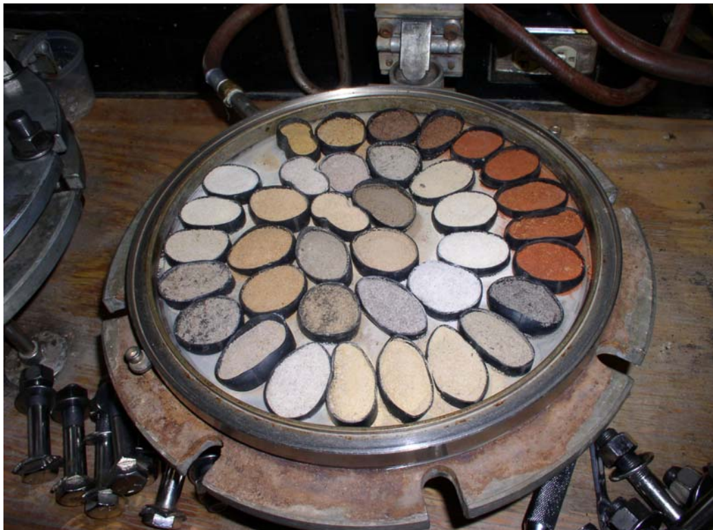
Figure 2. Pressure-membrane extraction at 1500-kPa for <2-mm samples.
