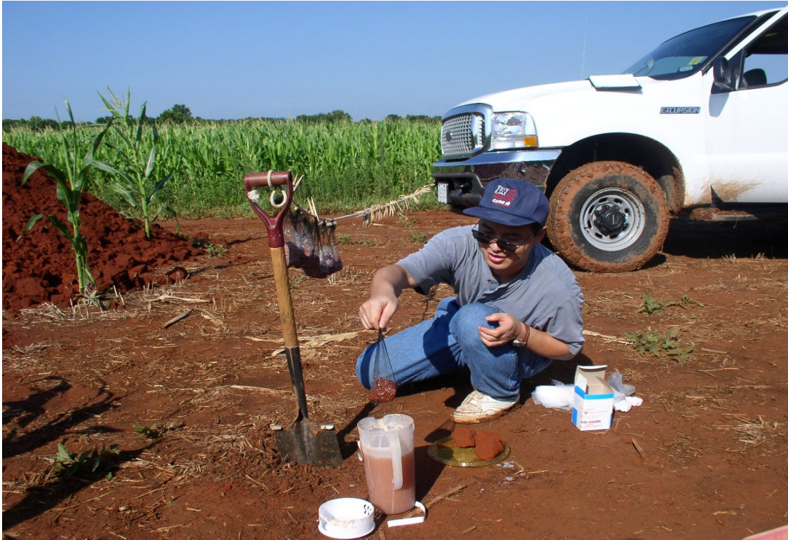
Fig. 1. Dipping clods with hairnet in plastic-lacquer.
