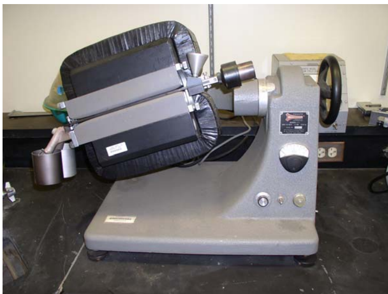
Fig. 1. Apparatus for Magnetic Separation
