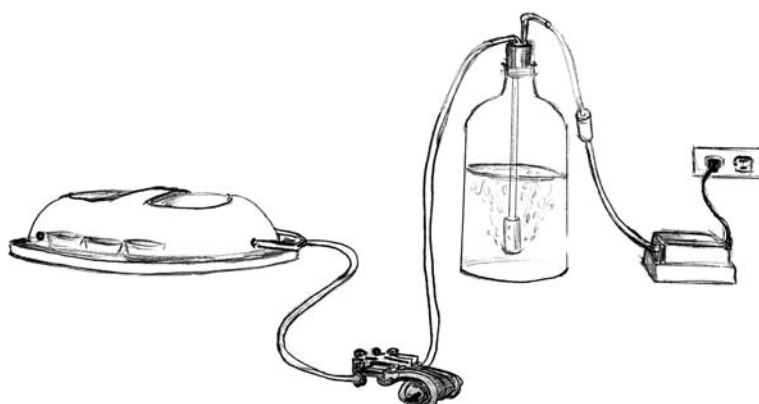
Fig. 1. Apparatus for measuring oxidized pH.
