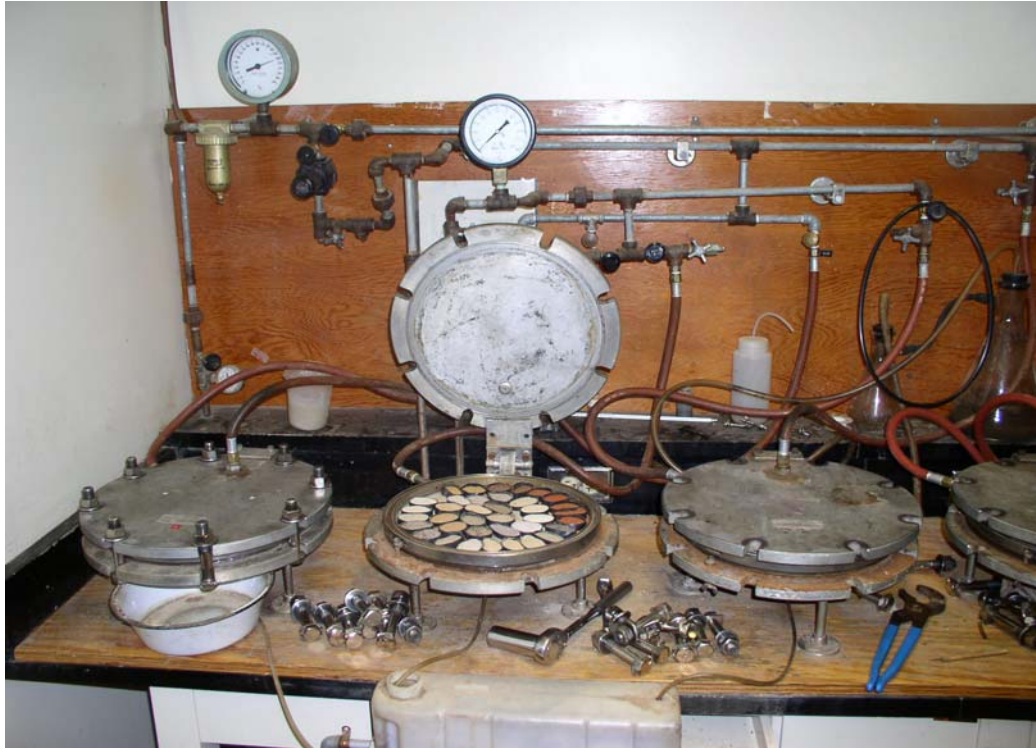
Figure 1. Sieved (<2-mm) soil placed in pressure-membrane extractor.
