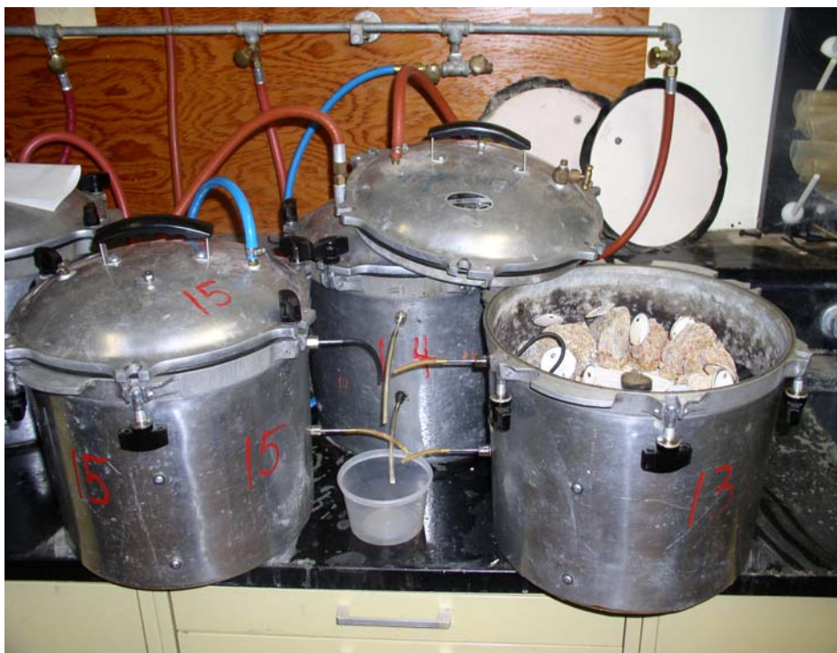
Fig 1. Clods placed in pressure-plate extractor following saturation.
