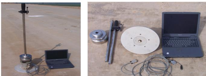
**FIG. 1. Portable Falling Weight Deflector**
