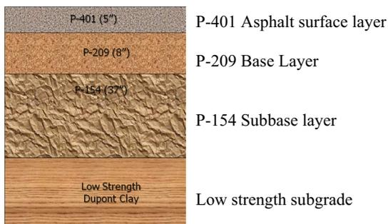
**FIG. 1. LFC Cross Section.**
